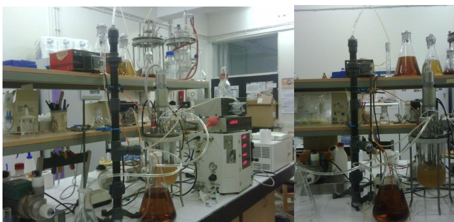
Figure 3.16 Fermentation Unit with Continuous Fresh Medium Feeding and Continuous Membrane Filtration (at the beginning of the experiment)
