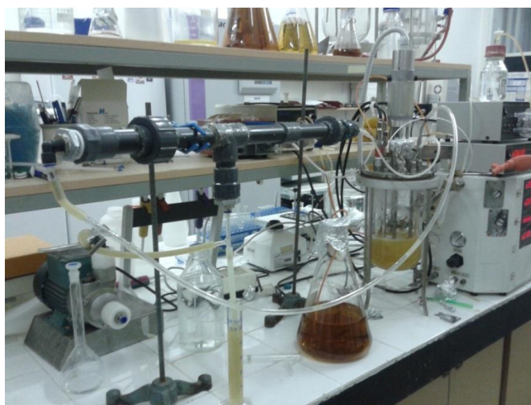
Figure 3.21 Membrane Bioreactor System Integrated to Fermentation Unit with Continuous Fresh Medium Feeding and Continuous Membrane Filtration, Backwashing System Incorporated
