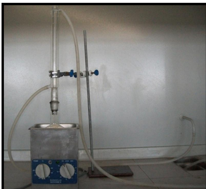
Figure 2.2 Oxidative Functionalization of Unmodified Carbon Nanotubes (CNTs) by Refluxing in an Ultrasonic Bath
