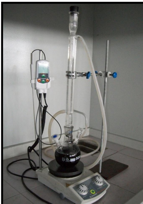
Figure 2.5 Aminosilanization of Oxidative Functionalized Carbon Nanotubes by Refluxing
