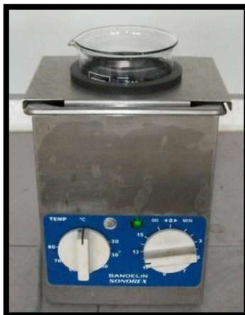
Figure 2.4 Ultrasonication of Oxidative Functionalized Carbon Nanotubes (f-CNTs) Before Aminosilanization
