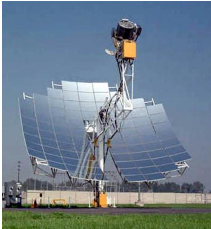
**Figure 1.8** Parabolic Dish [13]
