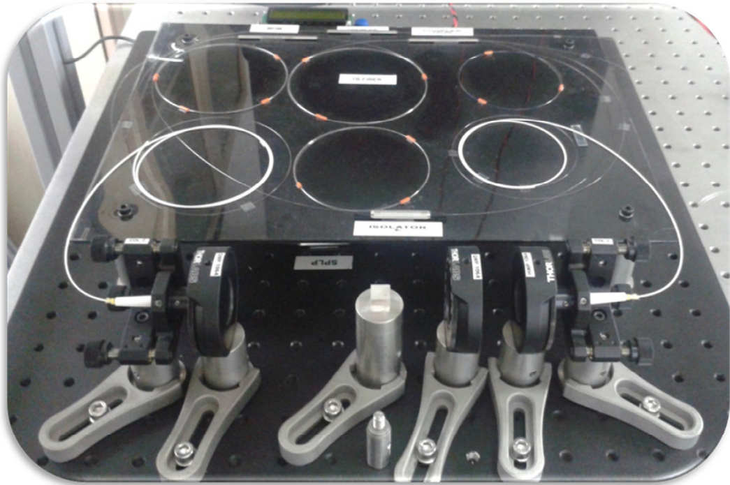
Figure 4.2 The photo of implemented mode locked Yb-doped fiber laser oscillator.
