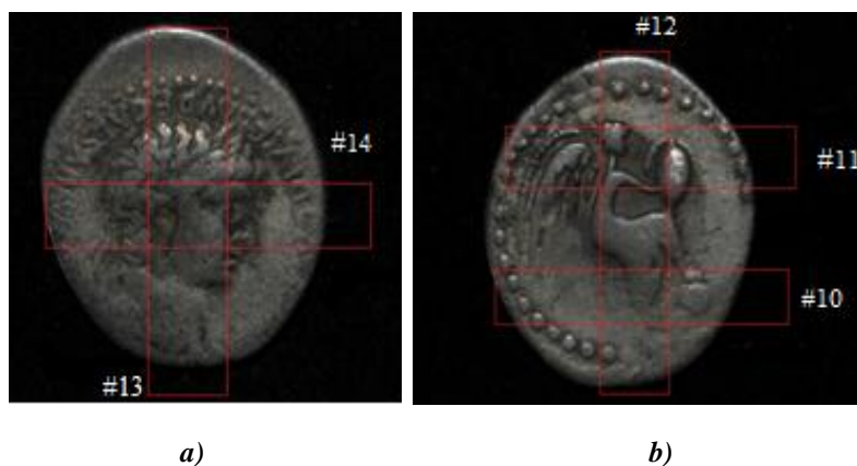
Figure 5.39: Use of pin hole with selected areas for P-XRF analysis of Claudius Hemi drachma, 150-870/15-76. a) Obverse b) Reverse.
