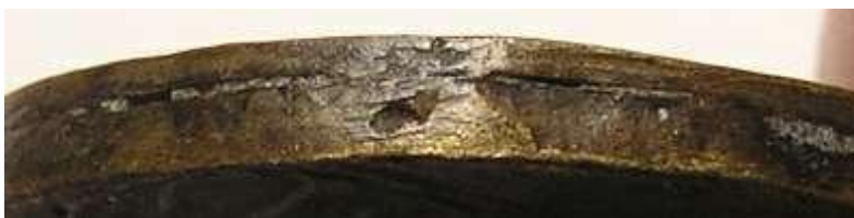
Figure 2.7: Joined shells trace of Electro types forgery ( http://www.calgarycoin.com/reference/fakes/electro.htm ).
