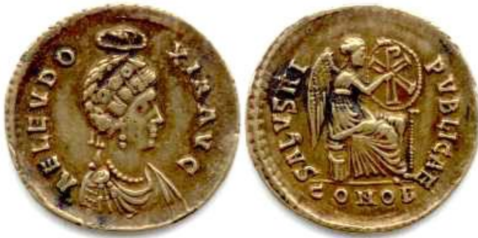
Figure 2.4: Fake coin made with lost/flying wax cast fake ( http://www.calgarycoin.com/reference/fakes/cast.htm ).
