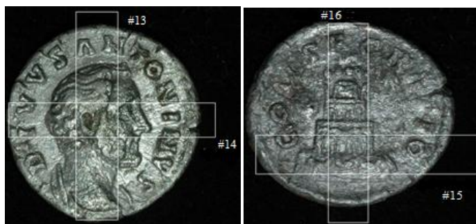
Figure 5.42: Use of pin hole with selected areas for P-XRF analysis of Antoninus Pius coin, 95-M190.
