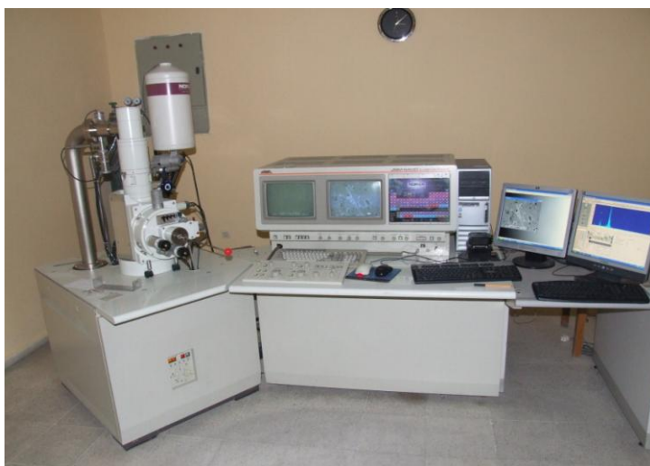
Figure 4.2: JSM 6400 SEMEDX Instrument used in the study.
