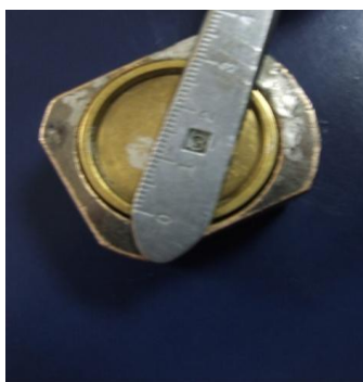
Figure 4.3: Sample holder of SEM with the size of 3cm in diameter.
