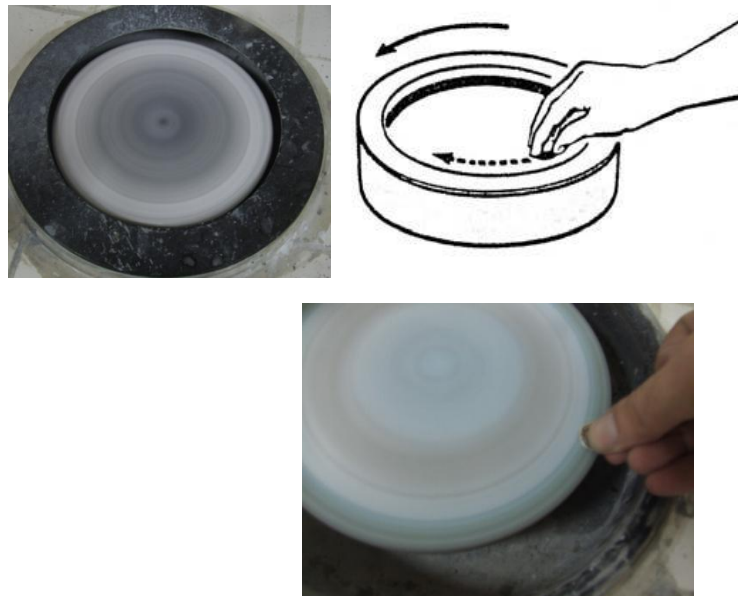
Figure 4.4 Polishing authentic and fake samples on the cleanest and flat part of them by using the rotary polishing wheels.
