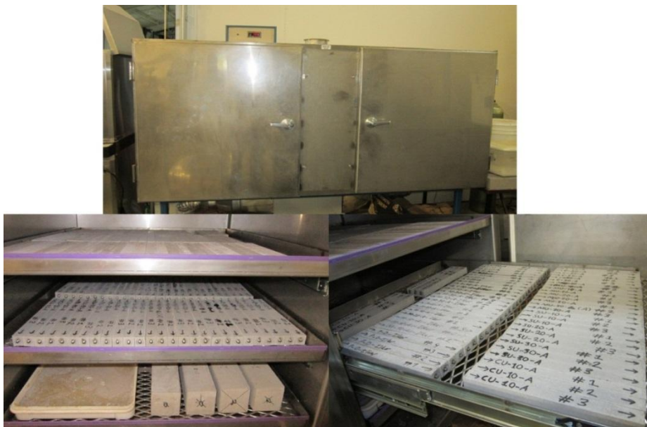
Figure 4. 18 The mortar bars stored in the drying room applicable to ASTM C157 (CAER Lab.)
