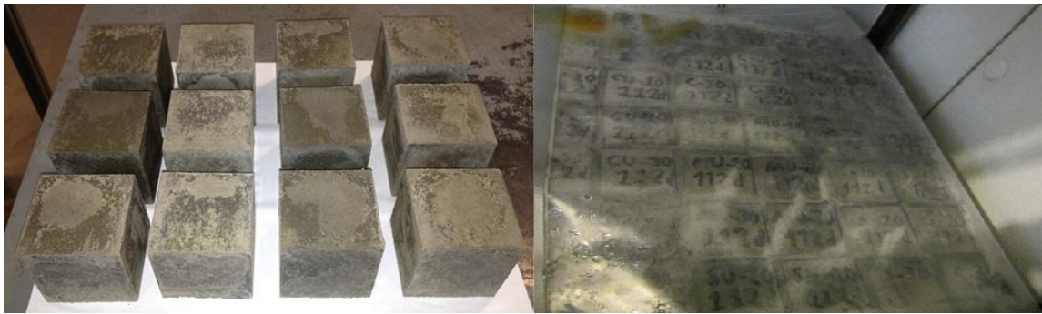
Figure 4. 14 The cubes after being removed from their molds (left) and in the moist room (right)
