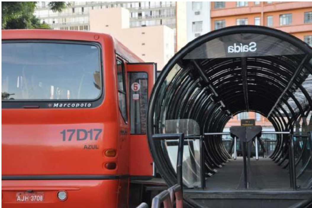
Figure 24: Station design of RIT, Curitiba, because of its physical configuration it is called tube station
