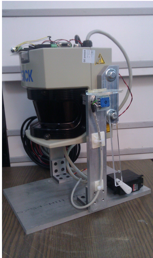
Figure 4.1: The mechanism which can rotate the sensor by an R/C servo and gets the information by a potentiometer.
