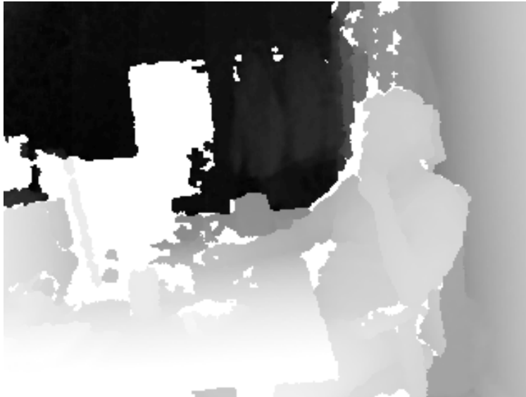
Figure 3.2: Capture of a person by Microsoft Kinect sensor. Bright areas are closer to the sensor than dark areas.
