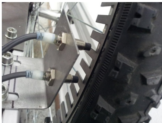
Figure 4.6: Proximity sensors and the encoder on the wheel.
