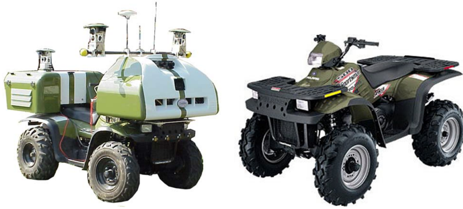
Figure 2.2: CyberATV, modified vehicle (left) and original vehicle (right).
