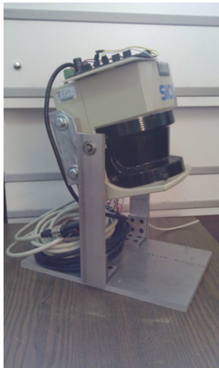
Figure 3.3: A simple apparatus to rotate Sick LMS291 around its X axis.
