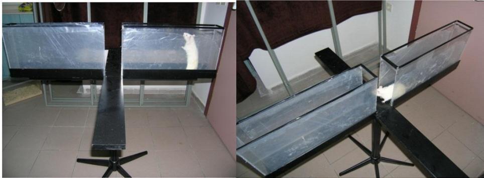
**Figure 2.4.** The Elevated Plus Maze Apparatus
