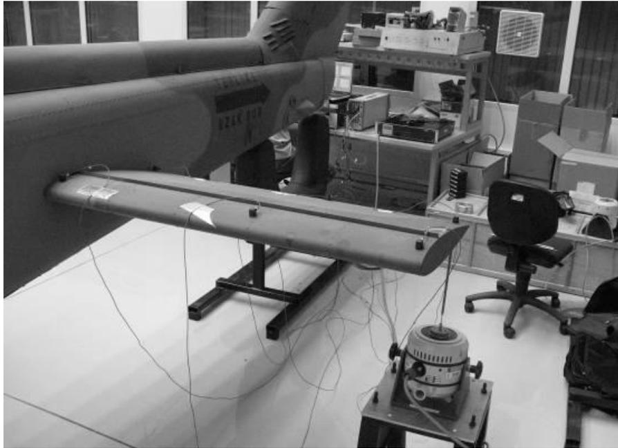
Figure 1-5. Modal tests performed on the horizontal stabilizer with testing equipment
