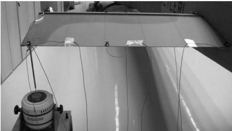
Figure 1-4. Modal tests performed on the horizontal stabilizer
