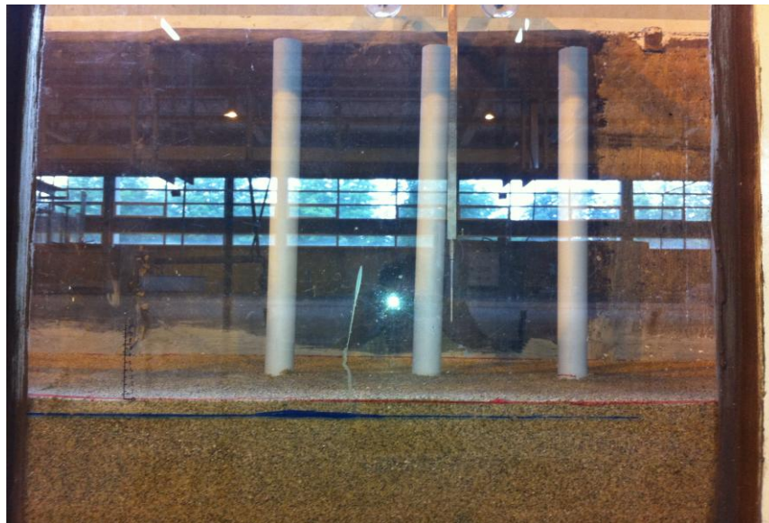
Figure C.2: 3 pier configuration ( D=50\text{mm} , \beta=0^\circ )
