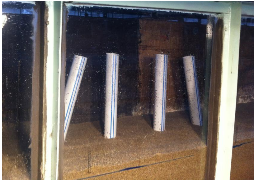
Figure C.1: 4 pier configuration ( D=70\text{mm} , \beta=10^\circ )
