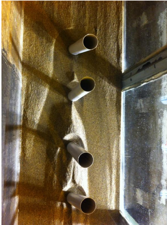
Figure C.3: Local scour formation after running the experiment (C2)
