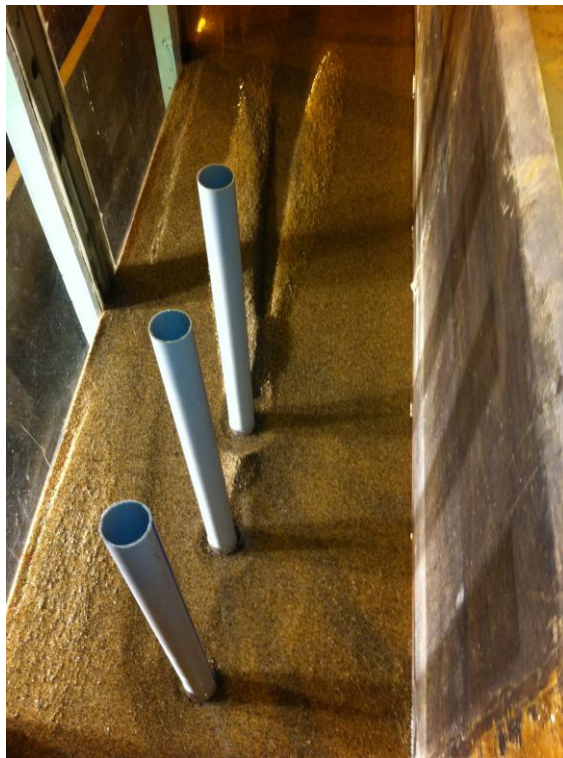
Figure C.4: Local scour formation after running the experiment (C1)
