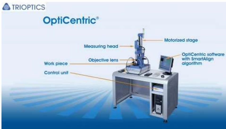
**Figure 36** Optical centering machine [31]
