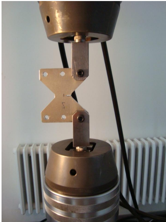
Figure 3. 14 Loading the specimen for fatigue precracking on MTS testing machine.
