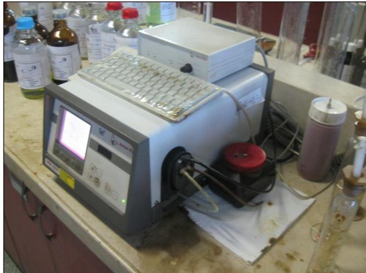
**Figure 5.8** Density meter used in experiments
