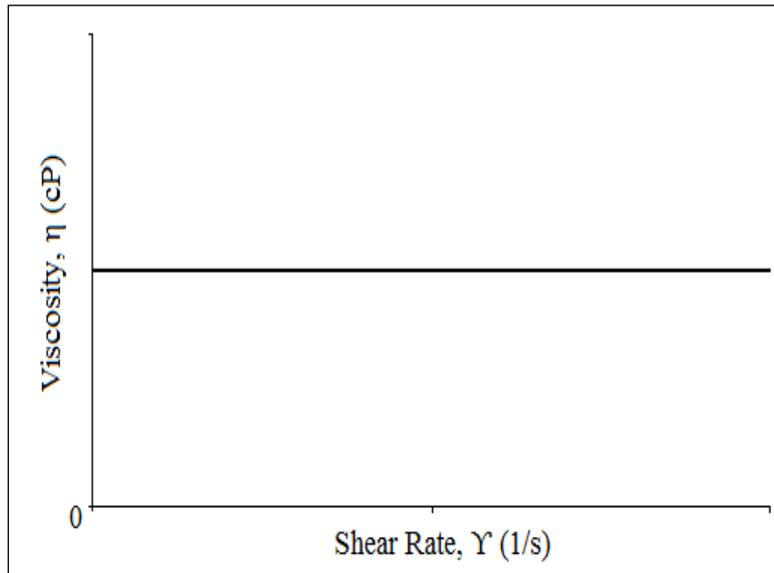
**Figure 4.11** Viscosity vs. Shear rate in Newtonian fluids [36].
