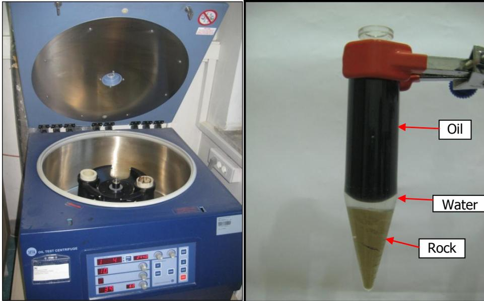
**Figure 5.6** Centrifugal separation of oil, water and rock mixture
