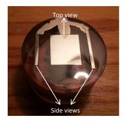
Figure 2-1 A representative sample for microstructural investigation.
