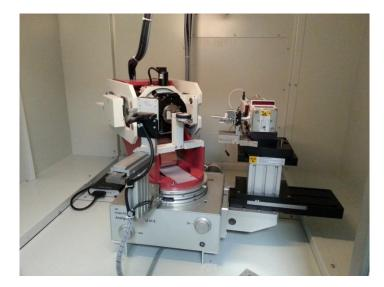
Figure 2-4 X-Ray system used in texture measurements
