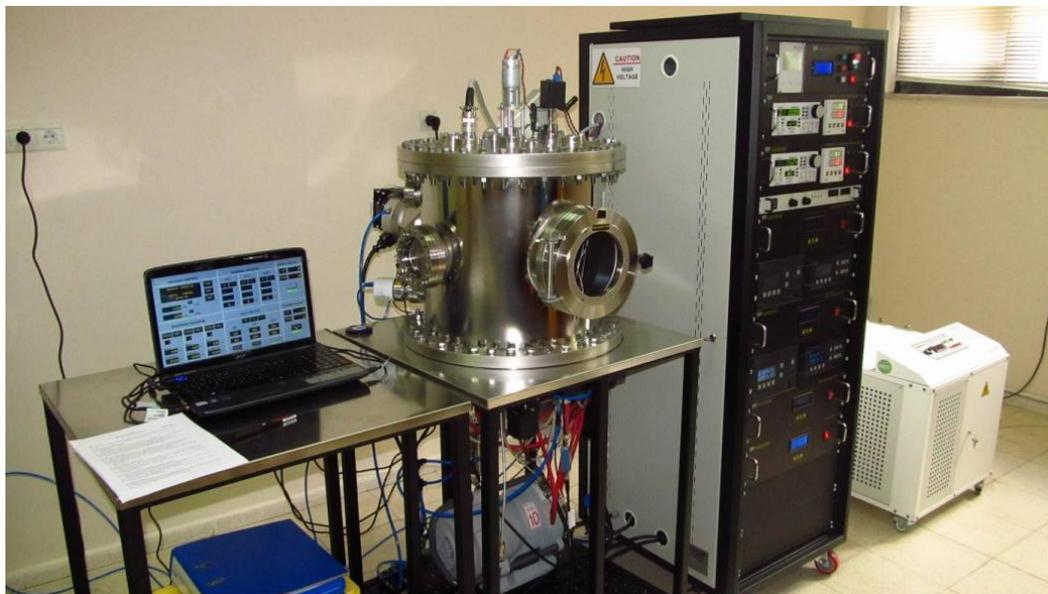
**Figure 3.1.** The view of Magnetron sputtering system.
