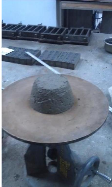
Figure 2.4 Flow table with the concrete mold removed.
