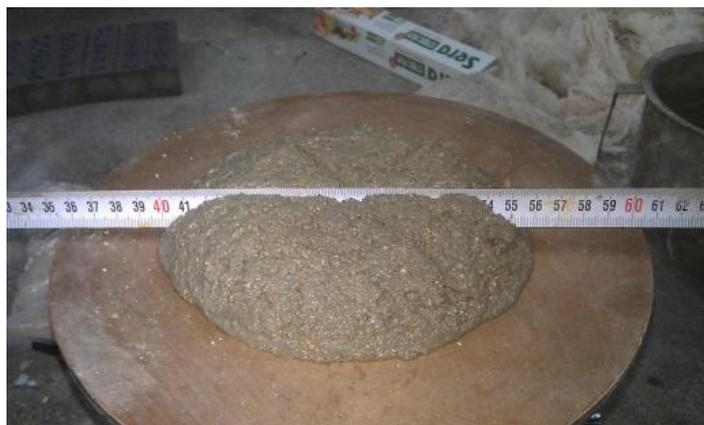
Figure 2.6 Concrete mixture with alkali lignin after flow, diameter measured.
