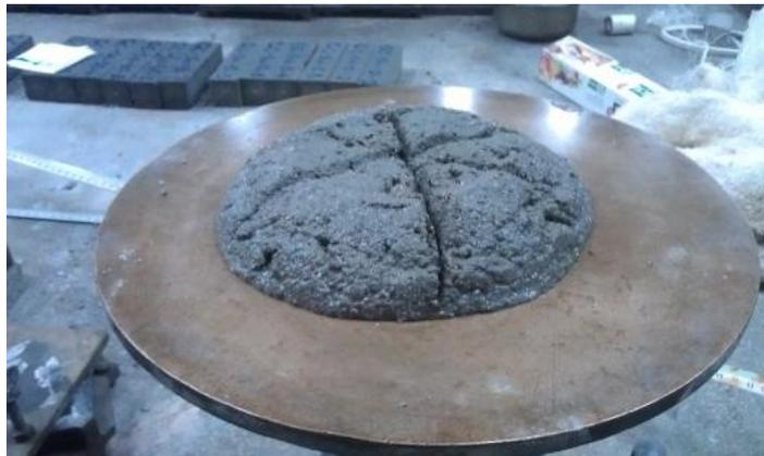
Figure 2.5 Control mix after flow.
