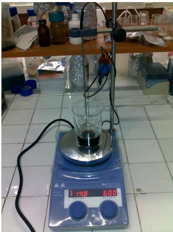
Figure 2.2 Experimental setup for the ionic liquid pretreatments.
