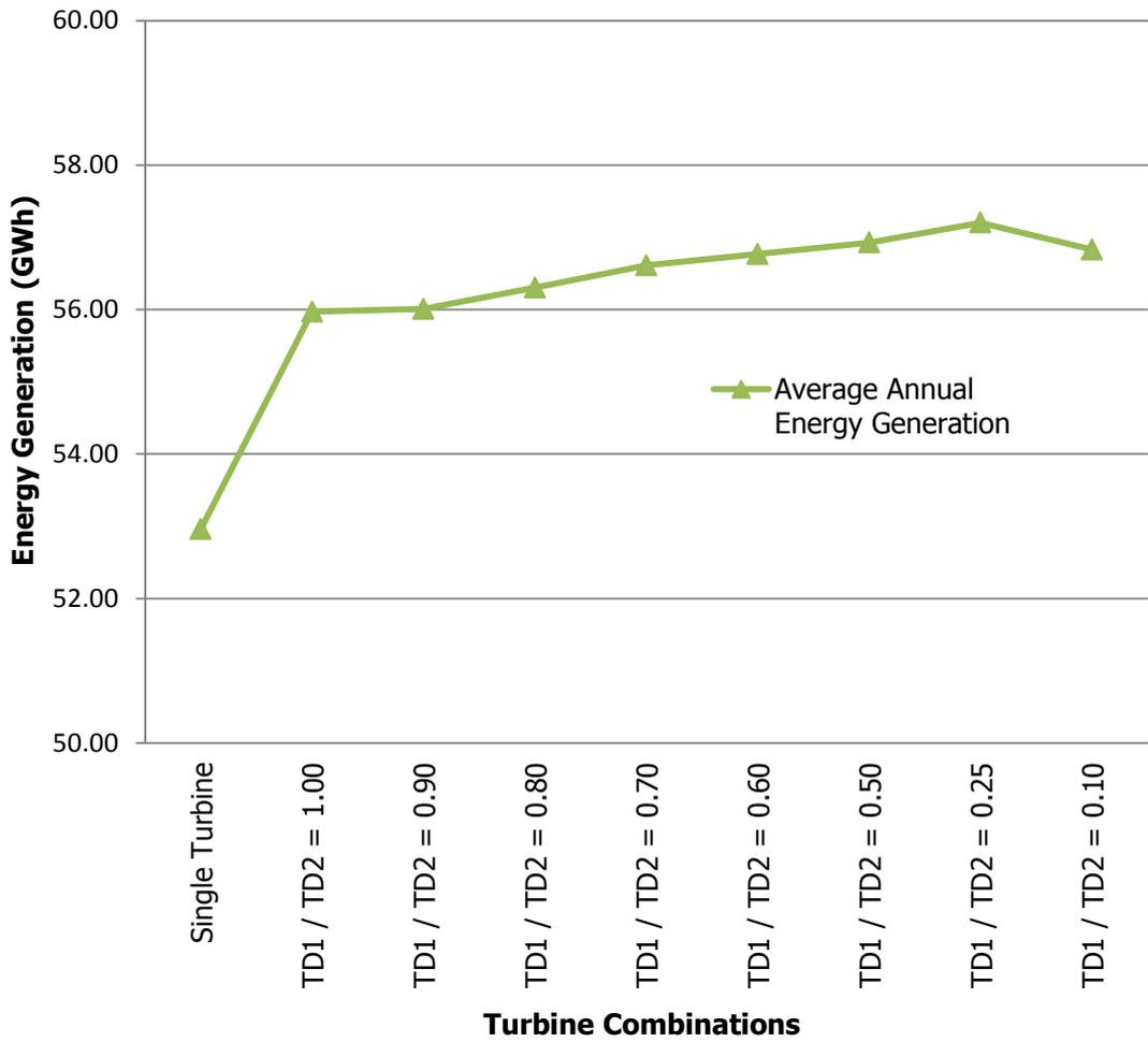
**Figure 3.16** The Change in Average Annual Energy Generation of the Discharge  $2.5 \text{ m}^3/\text{s}$  with respect to Different Turbine Combinations
