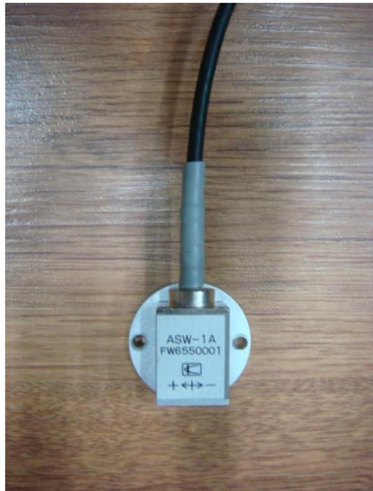
Fig. 3.19 ASW-1A accelerometer
