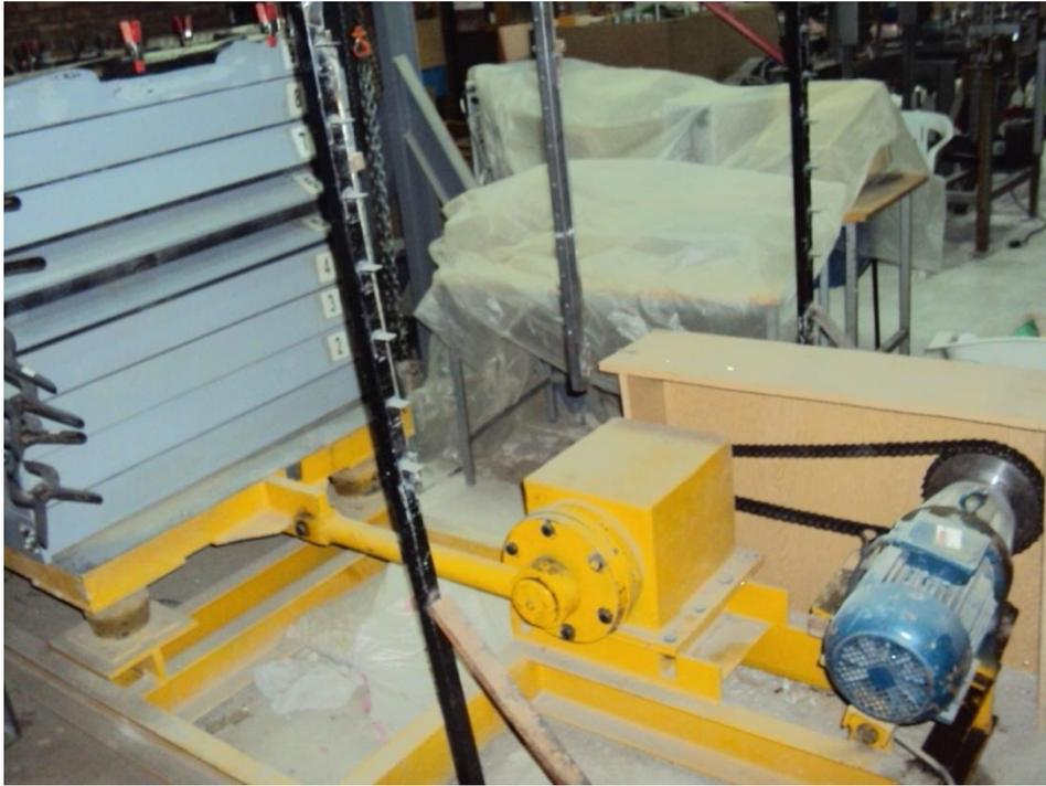
Fig. 3.1 The older shaking table, electric motor and gear system
