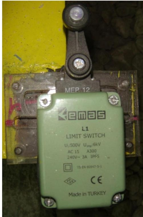
Fig. 3.9 The limit switch
