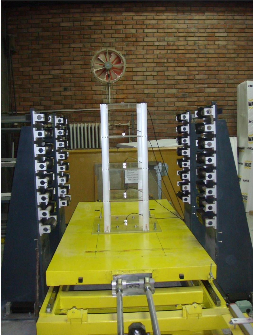
Fig. 3.25 A view of test setup for the 5-storey model (FB)
