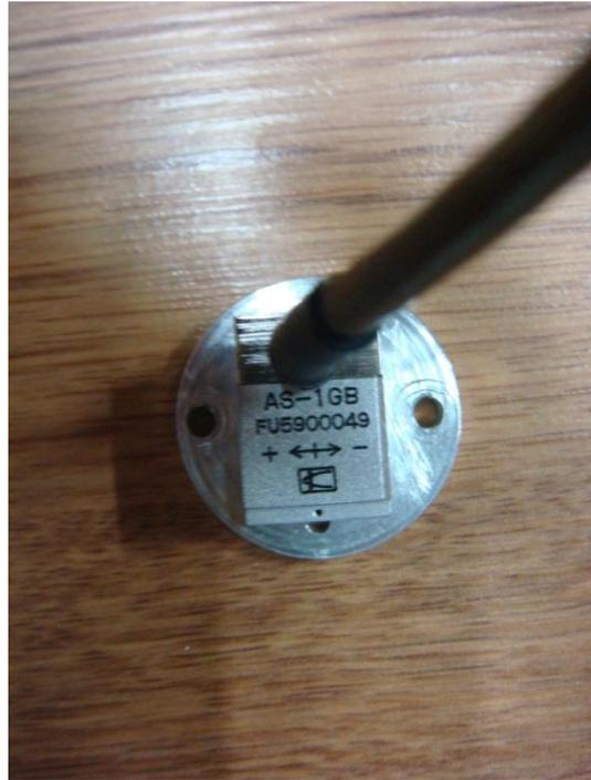
Fig. 3.18 AS-1GB accelerometer
