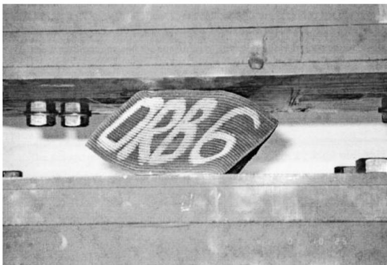
Fig. 2.18 The elastomer seismic isolator at failure (Kelly, 2002)
