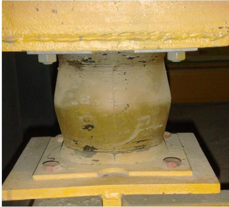
Fig. 3.11 Rubber bearings supporting the base in the older system
