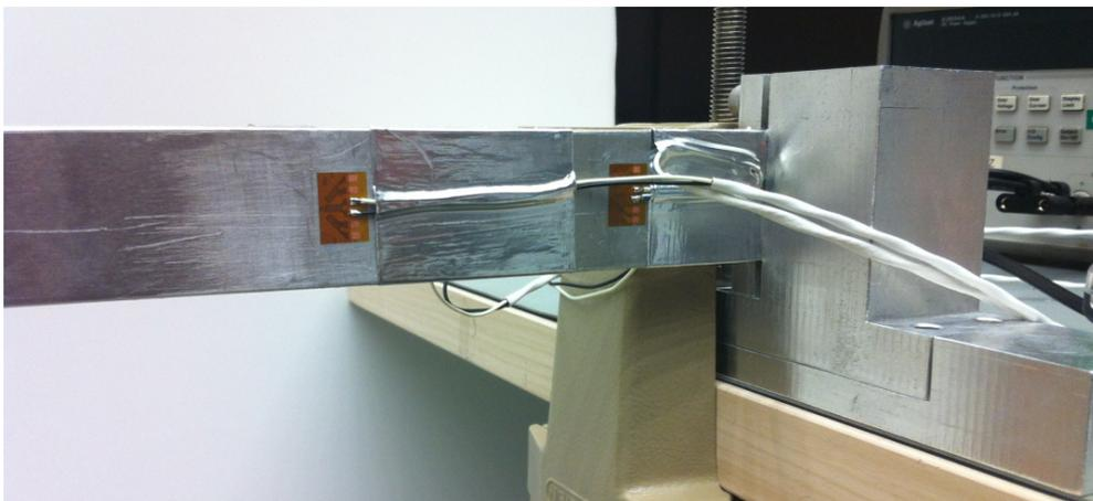
Figure 3-45 Picture of the bonded strain gages
