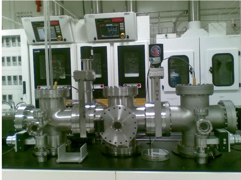
Figure 3.2: TUBITAK UME UHV-PECVD System
