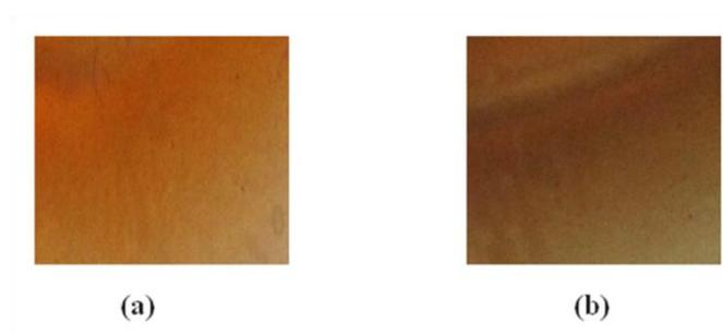
**Figure 3.13:** CHO /  $\text{Ph}_2\text{I}^+\text{PF}_6^-$  / PS1 mixture (a) before exposure to solar irradiation, and (b) after 5 minutes of exposure.
