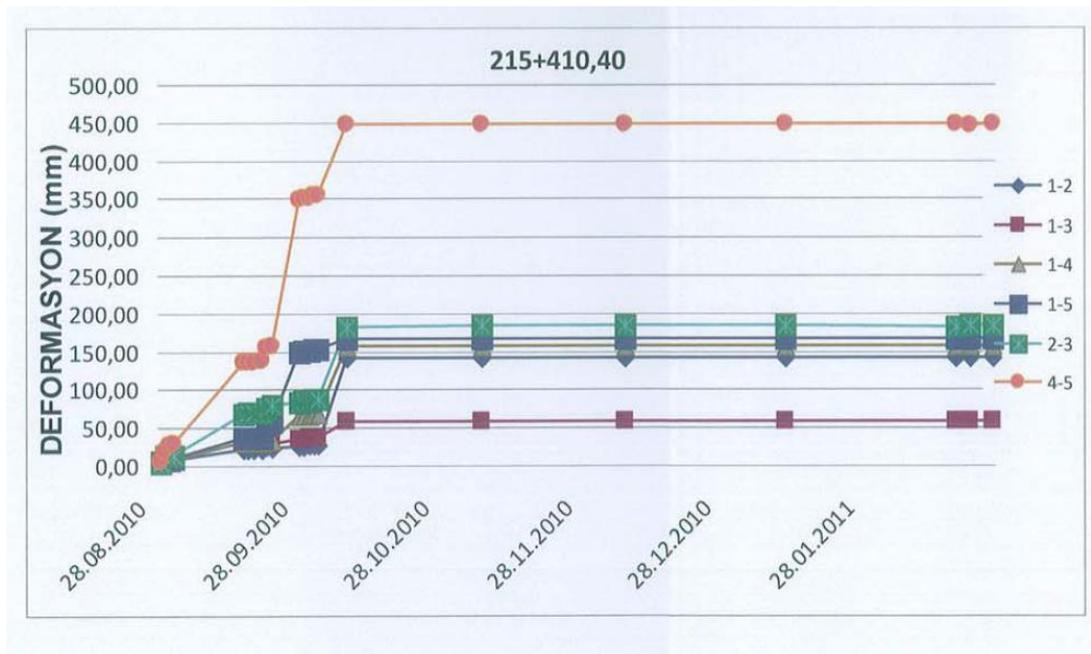
Figure 3.8 Deformation data of KM: 215+410 (after SIAL Report, 2011)
