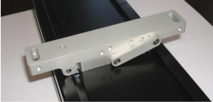
Figure 3.4: Laser beam positioning system mounting foot assembly
