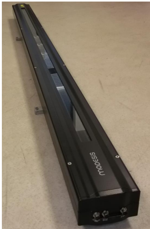
Figure 3.1: A photo of the laser beam positioning system (Model No: 2SH1S – 1800)
