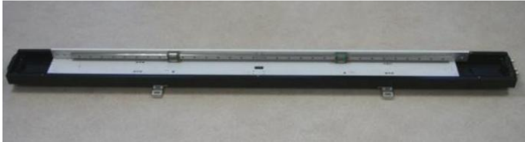
Figure 3.5: Laser positioning chassis, linear guideway, and carriages mounted to outer casing
