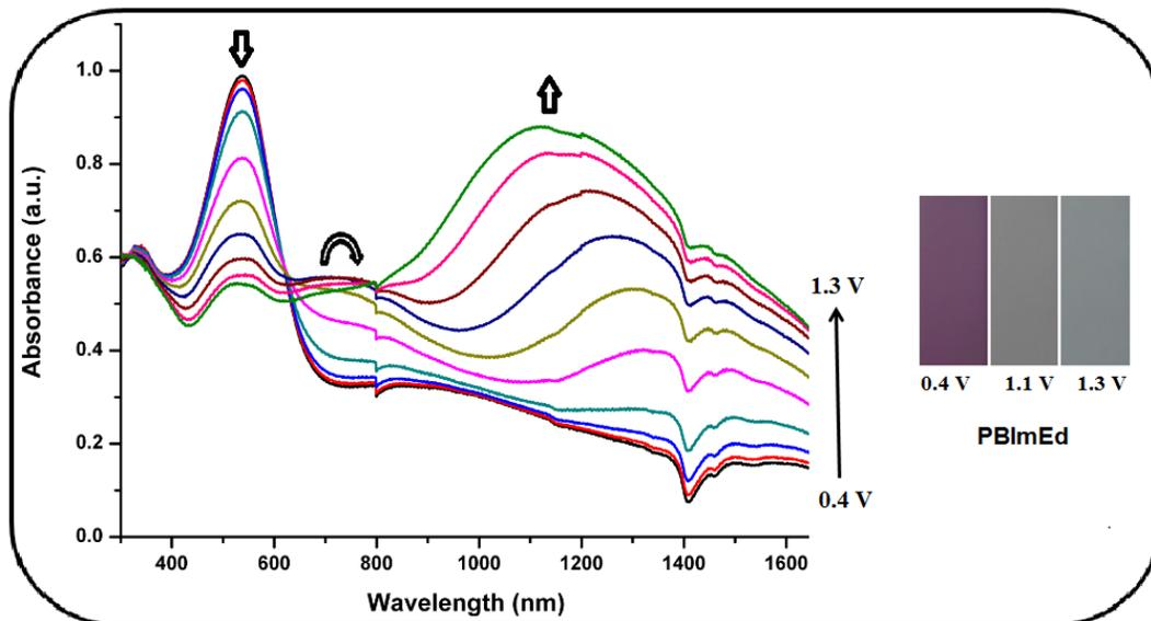
**Figure 3.13** Normalized absorption spectra of PBIImEd film on an ITO coated glass slide in monomer-free equimolar 0.1 M NaClO<sub>4</sub> and LiClO<sub>4</sub>, ACN solution upon doping between 0.4 V and 1.3 V with 0.1 V increments
