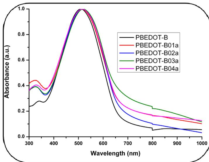
**Figure 5.14** Normalized vis spectra of PBEDOT-B, PBEDOT-B01a, PBEDOT-B02a, PBEDOT-B03a, PBEDOT-B04a in their reduced states
