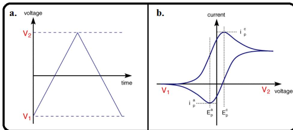
**Figure 2.10** a) Triangular waveform of cyclic voltammetry. b) Current-potential relation of a reversible redox process. Adapted from <http://www.ceb.cam.ac.uk/pages/linear-sweep-and-cyclic-voltammetry-the-principles.html>.
