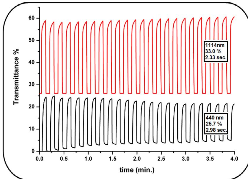
**Figure 3.14** Percent transmittance change of PBIImTh deposited on ITO electrode switching between 0.3 V and 1.2 V monitored at 440 and 1114 nm in monomer free equimolar 0.1 M NaClO<sub>4</sub> and LiClO<sub>4</sub>, ACN solution
