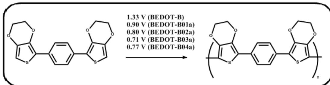
**Figure 4.5** Electrochemical polymerization of BEDOT-B in neutral and acidic conditions
