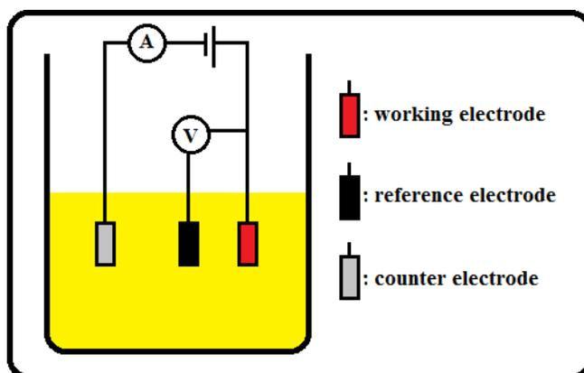
**Figure 2.9** Schematic representation of three electrode setup
