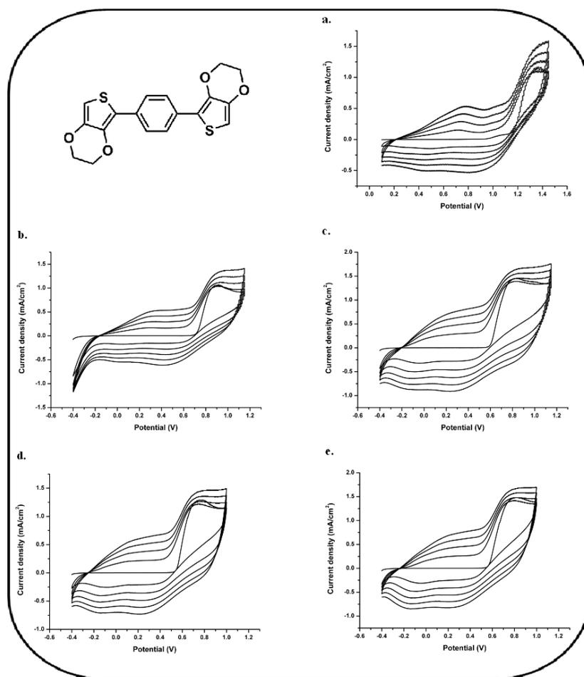
**Figure 5.9** Repeated potential scan of electrochemical polymerizations of (a) BEDOT-B, (b) BEDOT-B01a, (c) BEDOT-B02a, (d) BEDOT-B03a, (e) BEDOT-B04a in 0.1 M TBAPF<sub>6</sub>, DCM:ACN (5:95, v:v) with 100 mV/s scan rate
