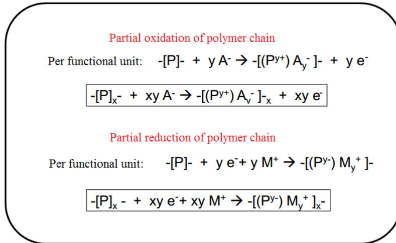
**Figure 1.4** Reactions occurring during partial oxidation and reduction of polymers.
