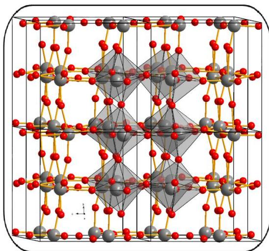
**Figure 1.2** Representative structure of tungsten (VI) oxide ( $\text{WO}_3$ ).
