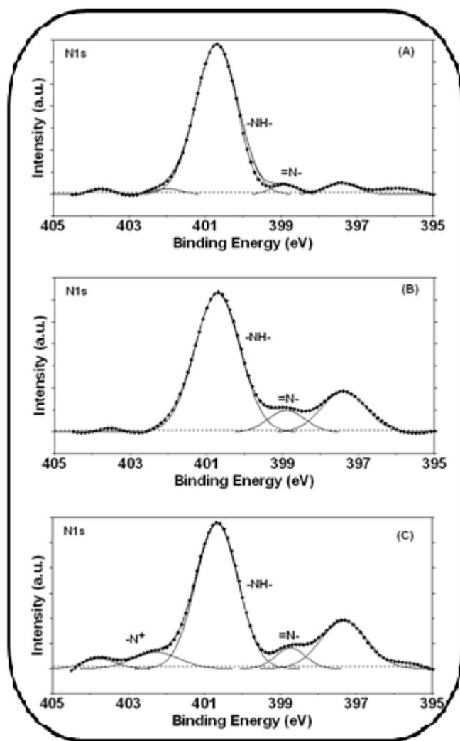
**Figure 5.8** N1s XPS data for (A) PBIImBEed, (B) PBIImBEed02b, and (C) PBIImBEed02a
