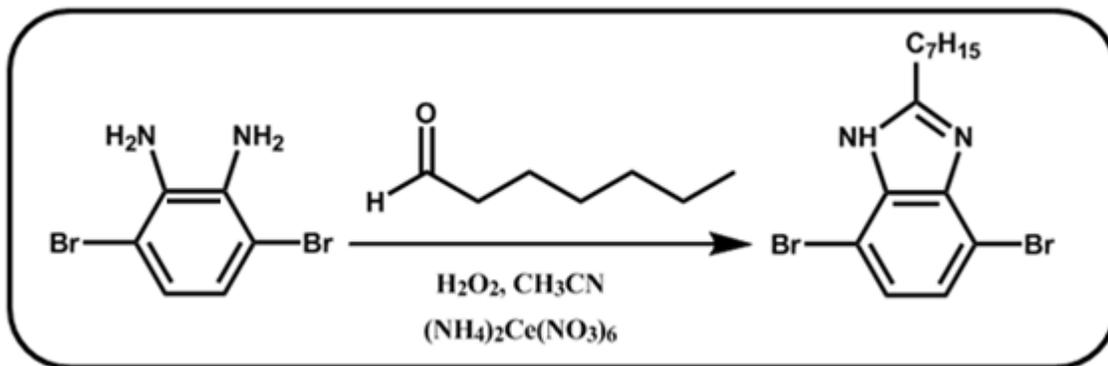
**Figure 2.3** Synthetic route for 4,7-dibromo-2-heptyl-1H-benzo[d]imidazole.
