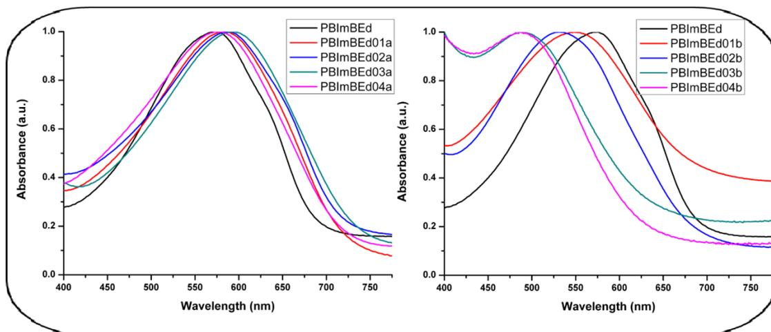
**Figure 5.13** Normalized vis spectra of PBImBE, PBImBE01a, PBImBE02a, PBImBE03a, PBImBE04a (left) and PBImBE, PBImBE01b, PBImBE02b, PBImBE03b, PBImBE04b (right) in their reduced states
