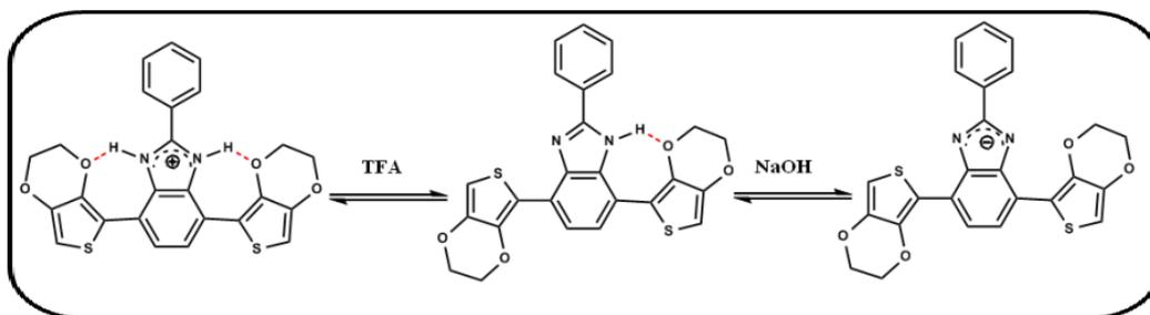
**Figure 5.7** Structures of BImBE<sub>d</sub> derivatives with acid and base addition
