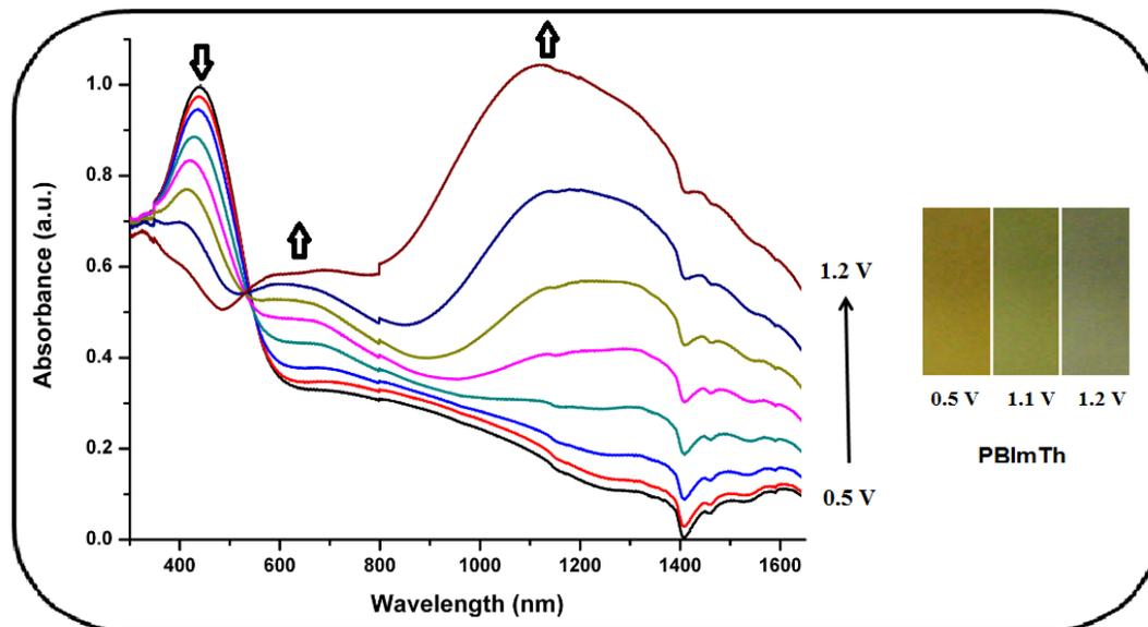
**Figure 3.12** Normalized absorption spectra of PBIImTh film on an ITO coated glass slide in monomer-free equimolar 0.1 M NaClO<sub>4</sub> and LiClO<sub>4</sub>, ACN solution upon doping between 0.5 V and 1.2 V with 0.1 V increments
