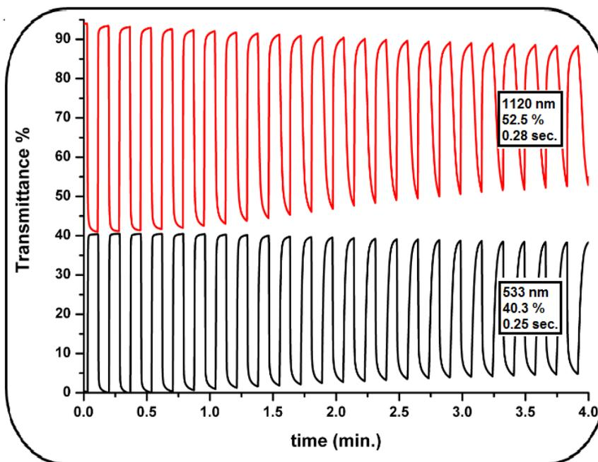
**Figure 3.15** Percent transmittance change of PBIImEd deposited on ITO electrode switching between 0.3 V and 1.3 V monitored at 533 and 1120 nm in monomer free equimolar 0.1 M NaClO<sub>4</sub> and LiClO<sub>4</sub>, ACN solution
