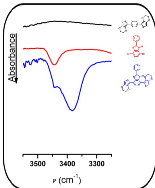
**Figure 5.5** FT-IR spectrum of BEDOT-B (up), 4,7-dibromo-2-phenyl-1H-benzo[d]imidazole (middle) and BImBEd (down) scanned in the amine stretching region in  $\text{CHCl}_3$  solution
