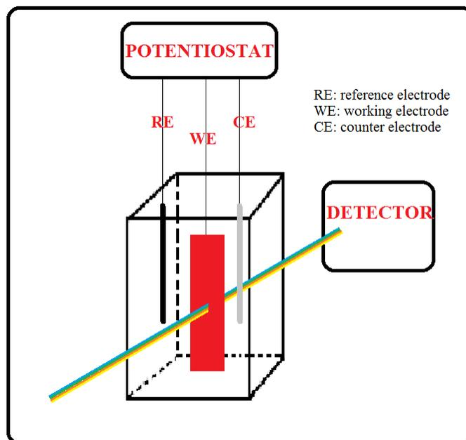
**Figure 2.12** Schematic representation of spectroelectrochemical instrumentation
