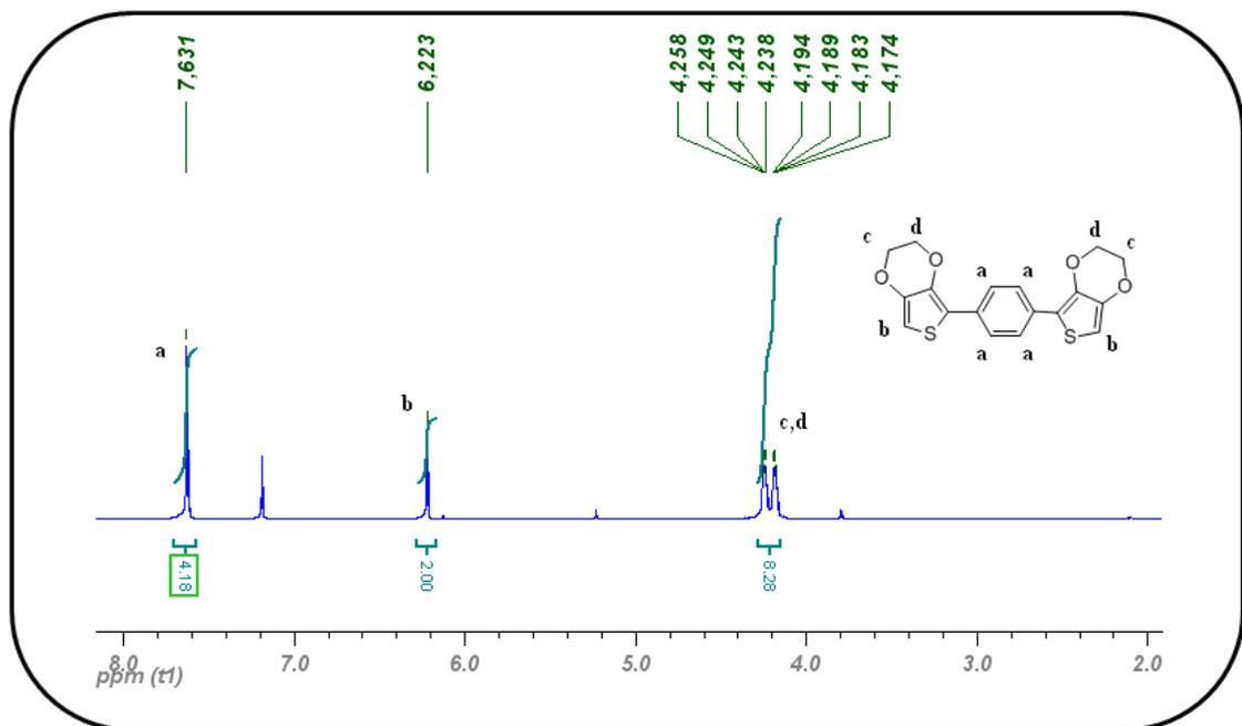
Figure 5.3  $^1\text{H}$ -NMR spectrum of BEDOT-B
