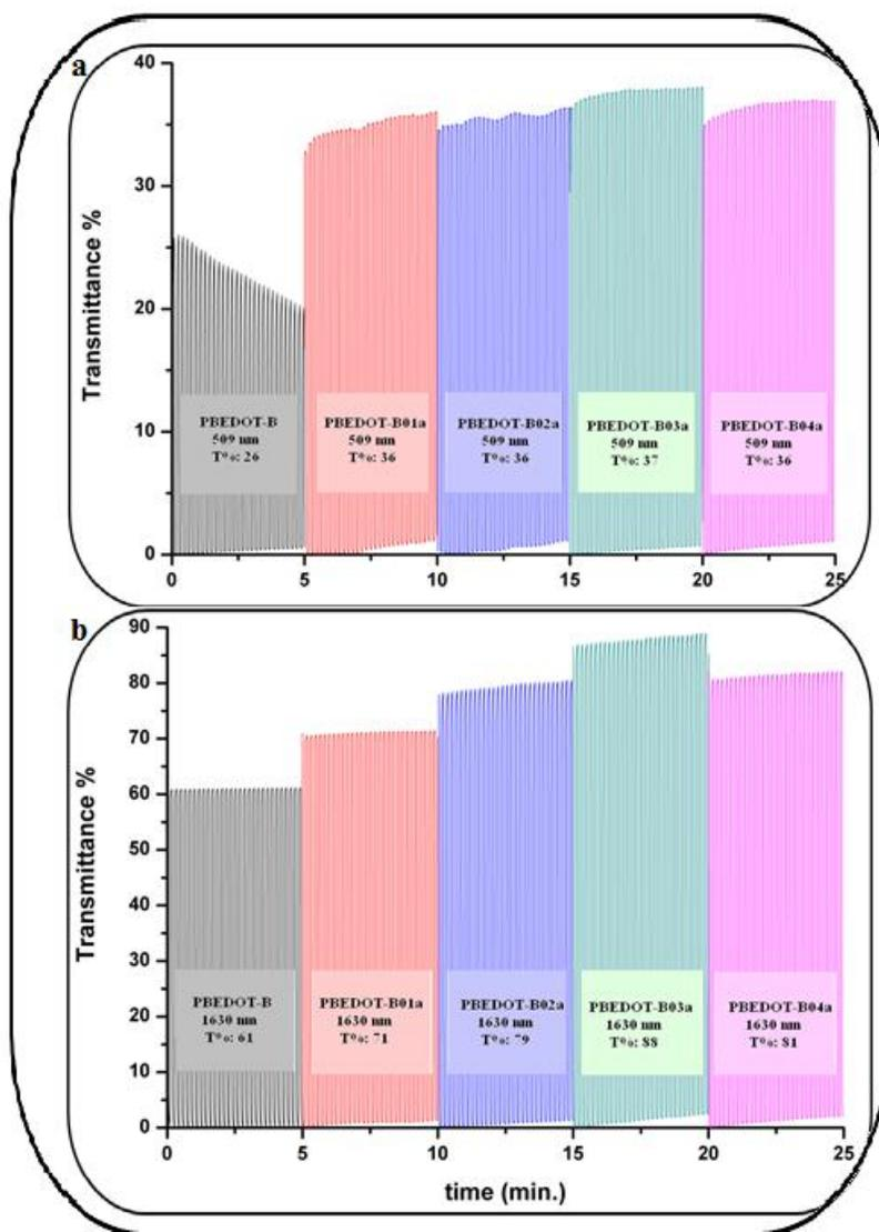
**Figure 5.17** Percent transmittance differences for BEDOT-B, BEDOT-B01a, BEDOT-B02a, BEDOT-B03a and BEDOT-B04a at their maximum absorption wavelengths in a) visible region, b) NIR region
