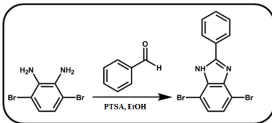
**Figure 4.1** Synthetic route for 4,7-dibromo-2-phenyl-1H-benzo[d]imidazole
