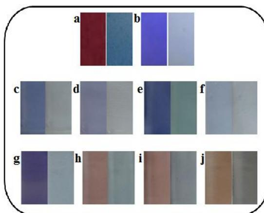
**Figure 5.15** Colors of the polymer films in their reduced (left) and oxidized (right) states for a) PBEDOT-B, b) PBI<sub>m</sub>BE<sub>d</sub>, c) PBI<sub>m</sub>BE<sub>d</sub>01a, d) PBI<sub>m</sub>BE<sub>d</sub>02a, e) PBI<sub>m</sub>BE<sub>d</sub>03a, f) PBI<sub>m</sub>BE<sub>d</sub>04a, g) PBI<sub>m</sub>BE<sub>d</sub>01b, h) PBI<sub>m</sub>BE<sub>d</sub>02b, i) PBI<sub>m</sub>BE<sub>d</sub>03b and j) PBI<sub>m</sub>BE<sub>d</sub>04b
