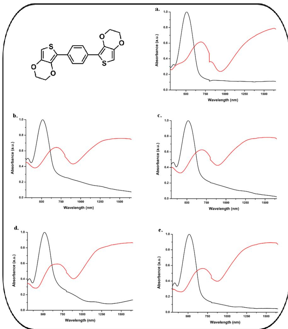
**Figure 5.12** Reduced (black lines) and oxidized (red lines) absorption spectra of (a) PBEDOT-B, (b) PBEDOT-B01a, (c) PBEDOT-B02a, (d) PBEDOT-B03a, (e) PBEDOT-B04a
