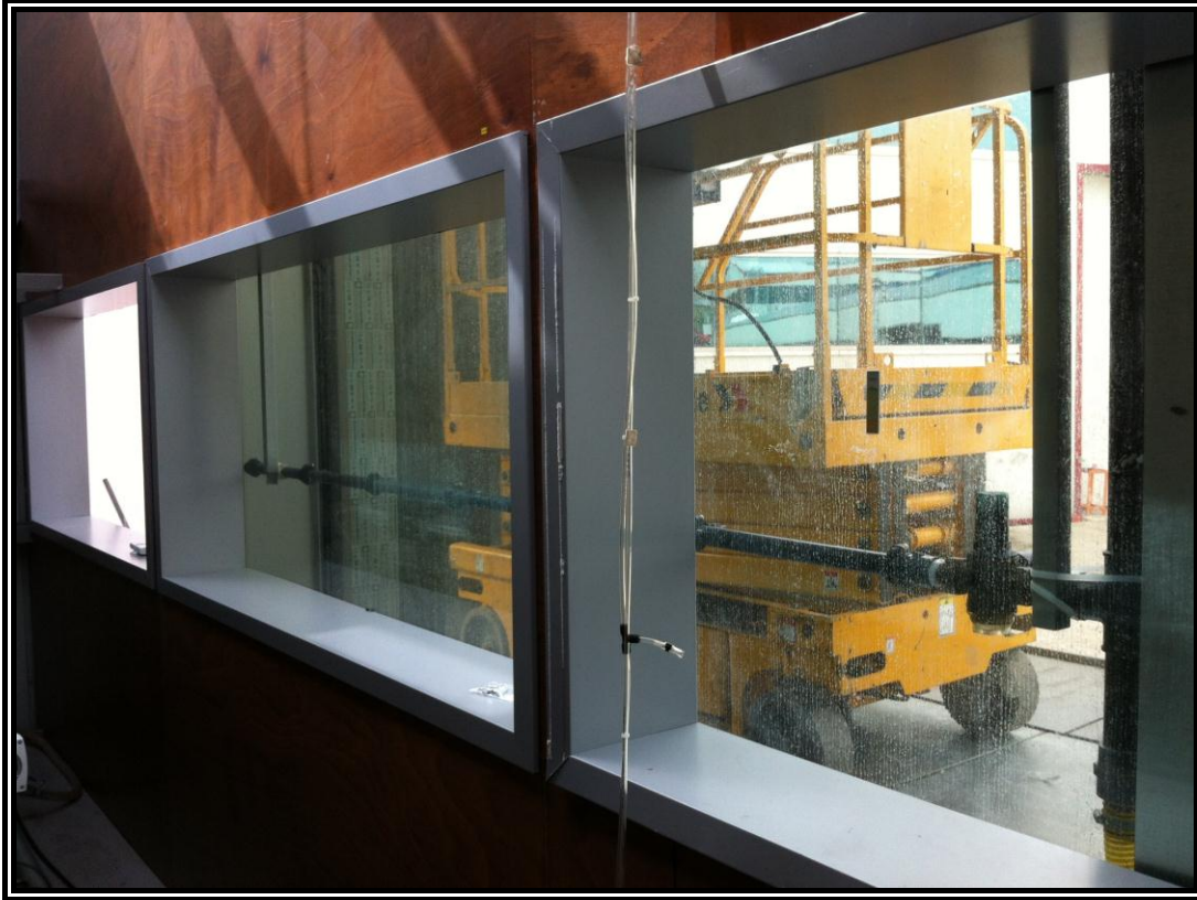
Figure 4.5 The View from The Watertightness Laboratory Test Under Static Pressure (Source: Individual Archive of The Author, 2012)
