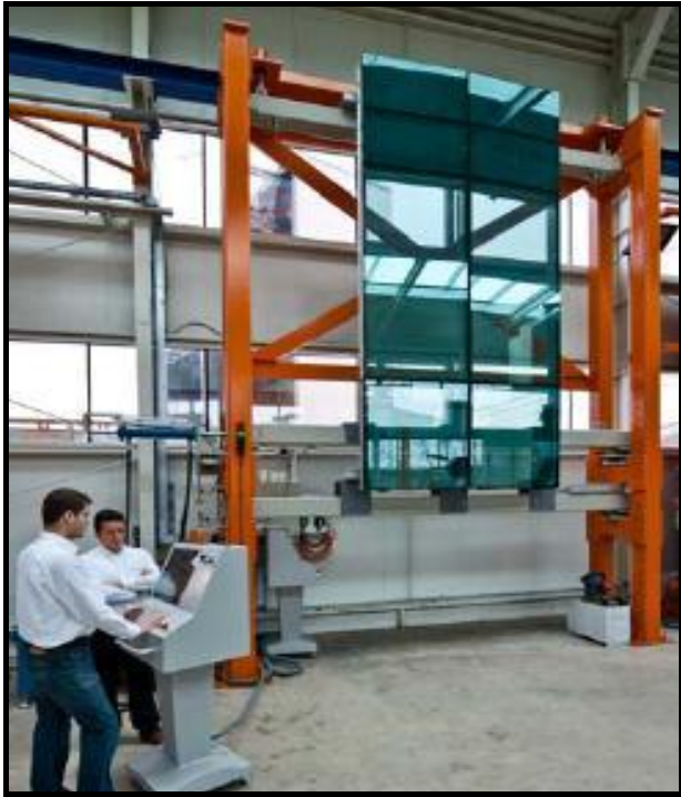
Figure 2.55. The View From Dynamic Building Movement Test (Source: http://fti-europe.com , Retrieved November, 2012)
