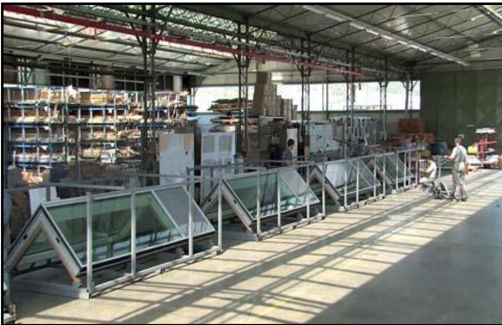
Figure 2.26. The Preassembled Units of Unitized Curtain Wall System (Source: Metal Yapı, 2012)
