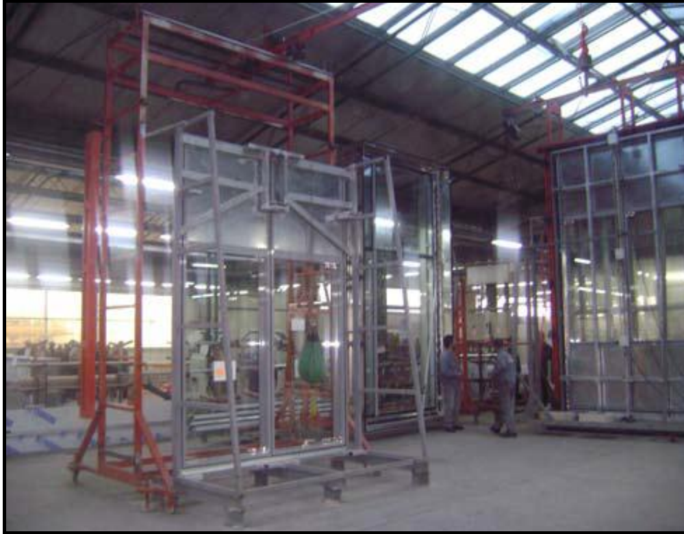
Figure 2.25. The Preassembled Units of Unitized Curtain Wall System (Source: Metal Yapı, 2012)
