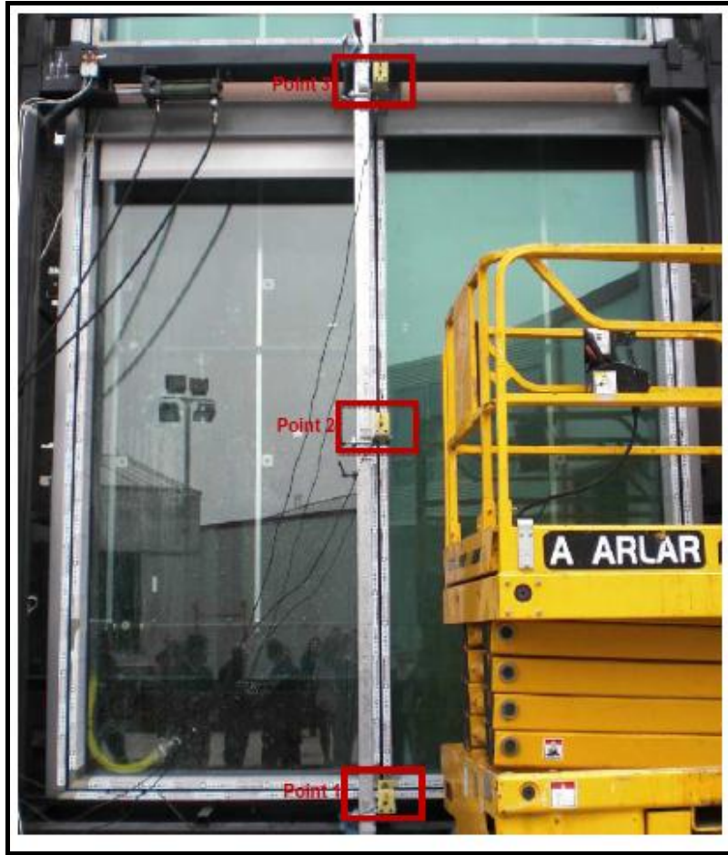
Figure 4.6. Three Position Sensors Placed on the Vertical Member
