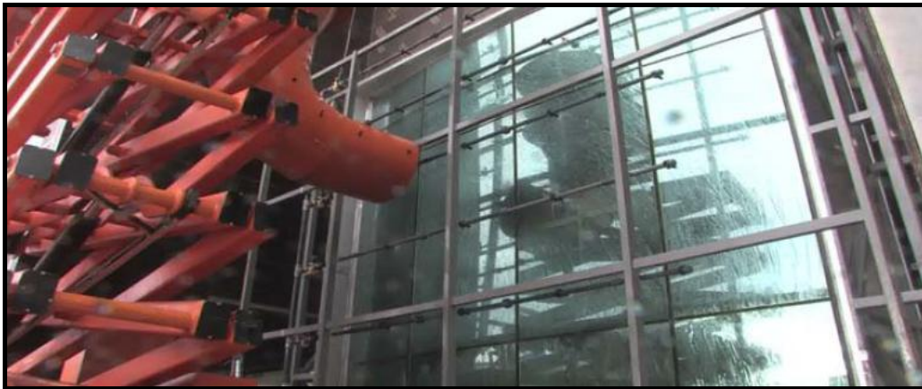
Figure 2.49. The Photo Taken from The Dynamic Air Permeability and Water Spray Test (Source: http://fti-europe.com , Retrieved November, 2012)
