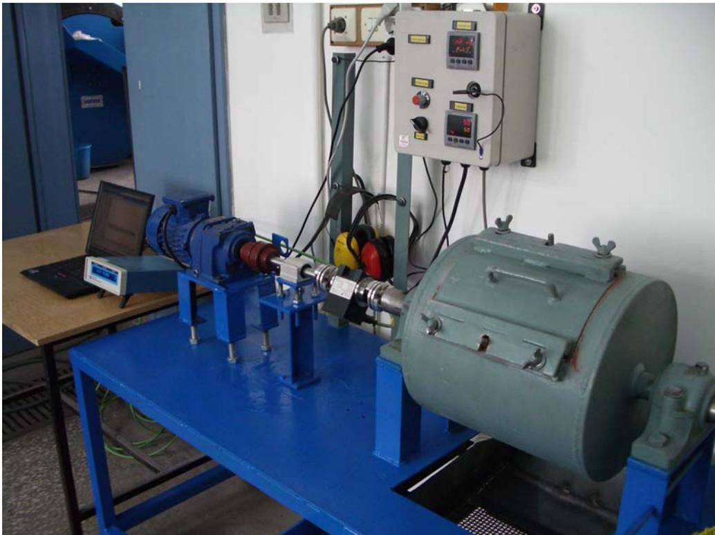
Figure 3.2. The picture of Bond Mill set-up
