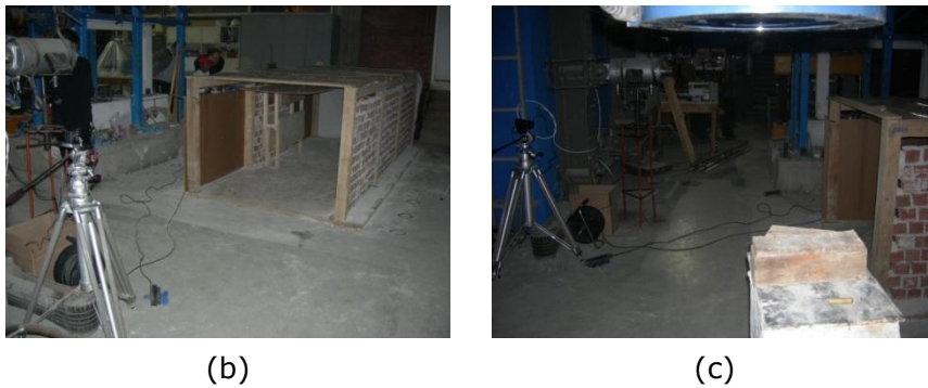
Figure 4.20 (a) Sketch and (b, c) photographs of the video camera monitoring the wide corridor model
