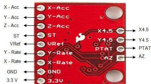
Figure 3.10 The back view of the IMU 5 DOF sensor with input and output pins
