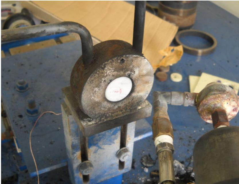
**Figure 40: Teflon Specimen on the Test Set-Up**
