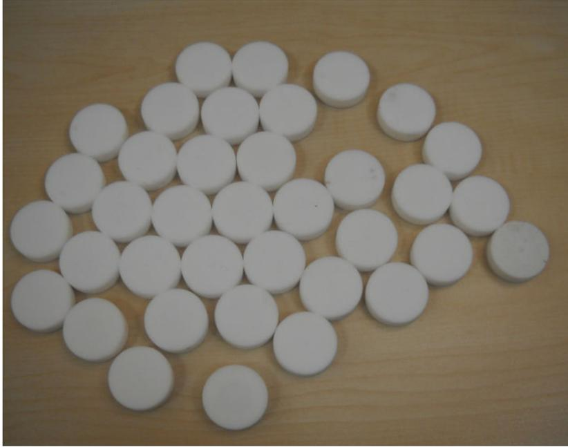
**Figure 39: Teflon Specimens Used for Oxyacetylene Tests**
