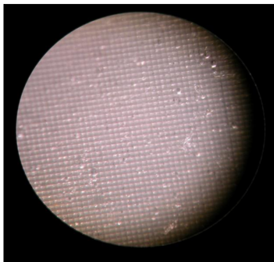
Figure 3.17: Stereomicrograph of multilayer scaffold with 4 layers of UXL Col film. Magnification: x45.
