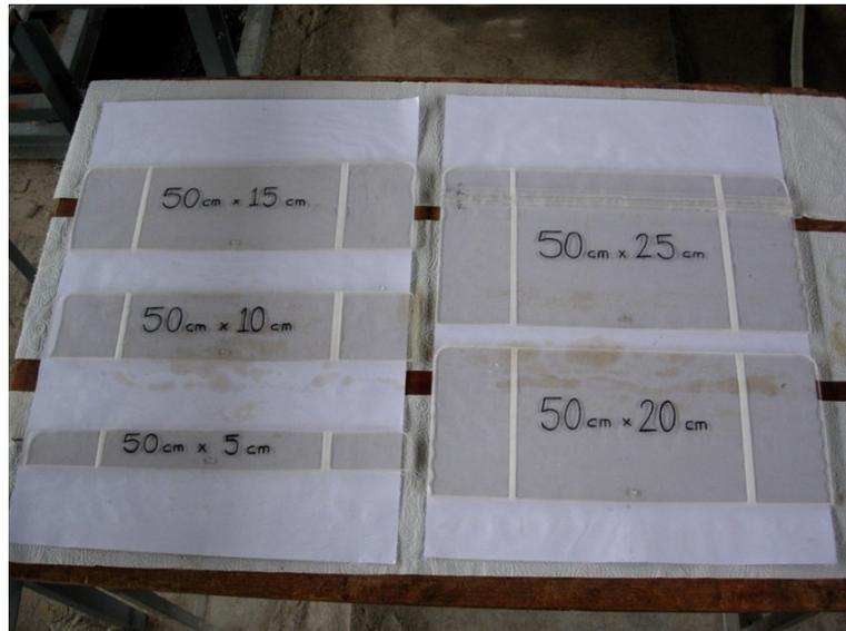
Figure 4.7 Anti – vortex plates with 50 cm in length
