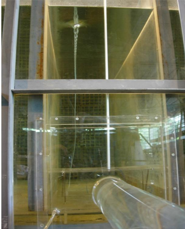
Figure 4.9 View of an air-entraining vortex forming at higher submergence
