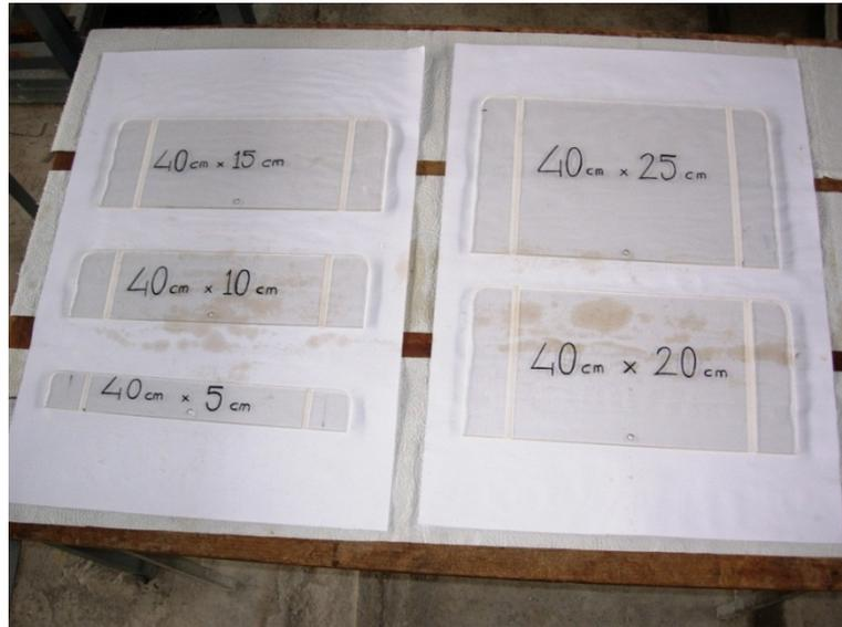
Figure 4.6 Anti – vortex plates with 40 cm in length
