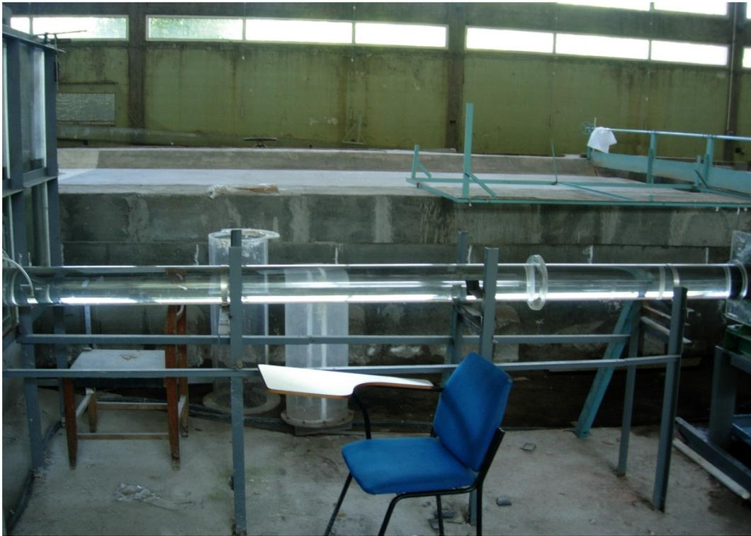
Figure 4.4 Experimental setup with intake pipe of  $D_i = 14.4$  cm
