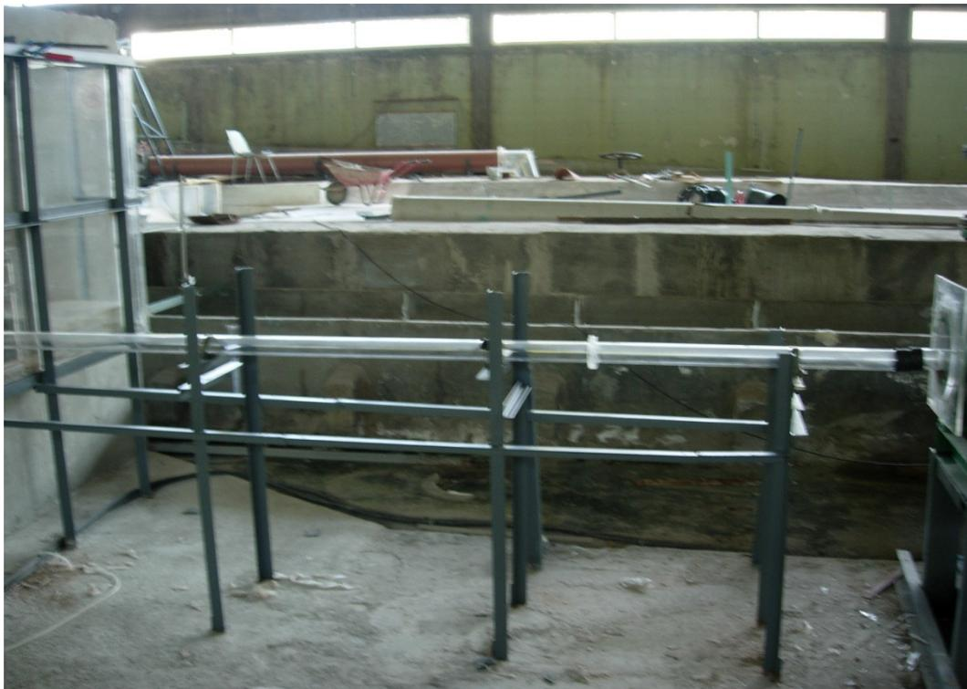
Figure 4.5 Experimental setup with intake pipe of  $D_i = 5$  cm
