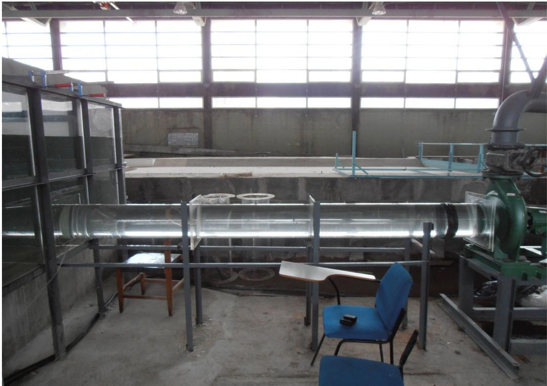
Figure 4.3 Experimental setup with intake pipe of  $D_i = 25$  cm
