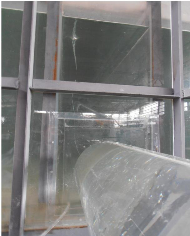
Figure 4.10 Vortex formation at the pipe of  $D_i = 25$  cm
