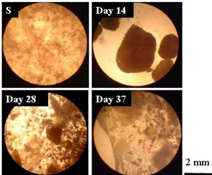
Figure 4.6 Microscopic view of sludge in R2 in Set-1 (S: Seed Sludge)
