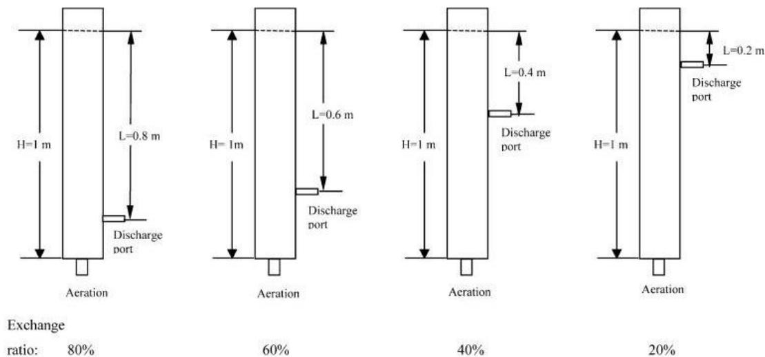
Figure 2.2 Different Exchange Ratios (L/H) of SBR (Liu et al., 2005c)
