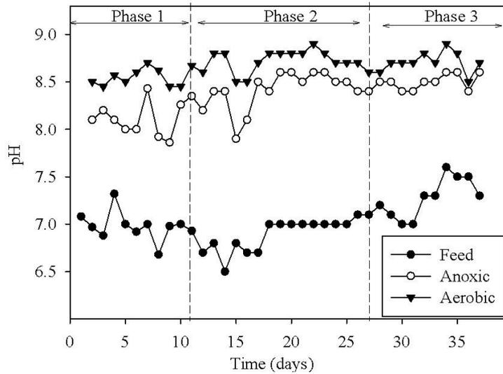
Figure 4.2 pH variations of R2 during operation (CAS) in Set-1 (-○- anoxic period -▼- aerobic period)
