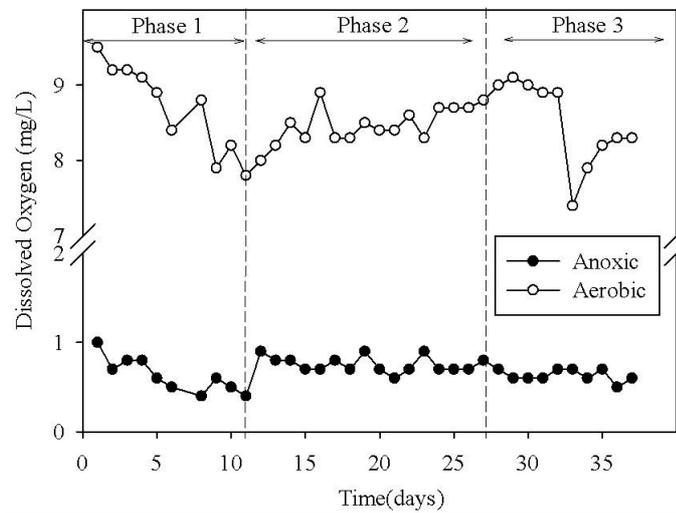
Figure 4.3 DO concentrations in R1 during operation in Set-1 (-●- anoxic period -○- aerobic period)
