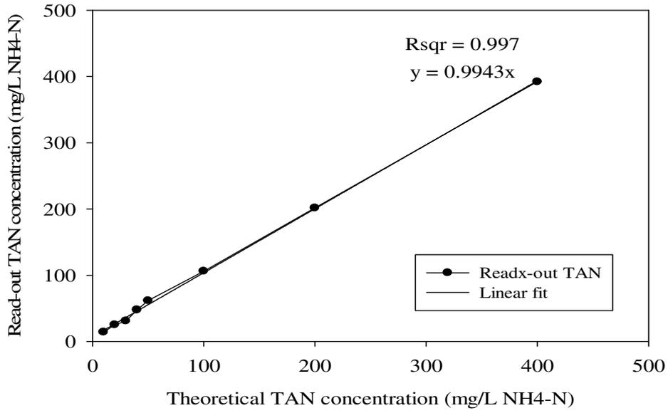
Figure B. 3 Calibration curve for TAN range of 10-400 mg/L
