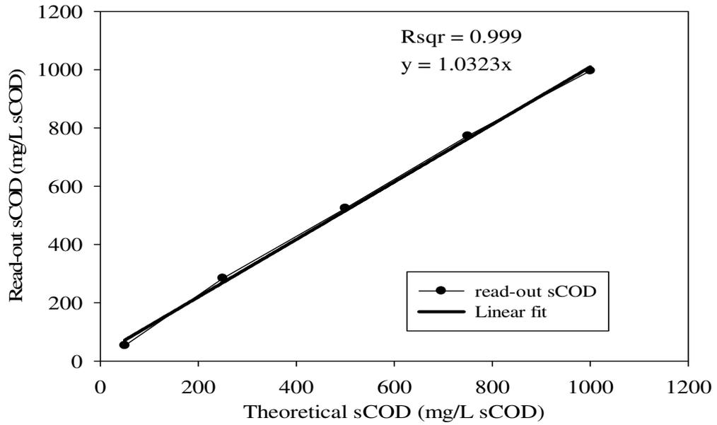
Figure B. 1 Calibration curve for sCOD range of 0-1500 mg/L
