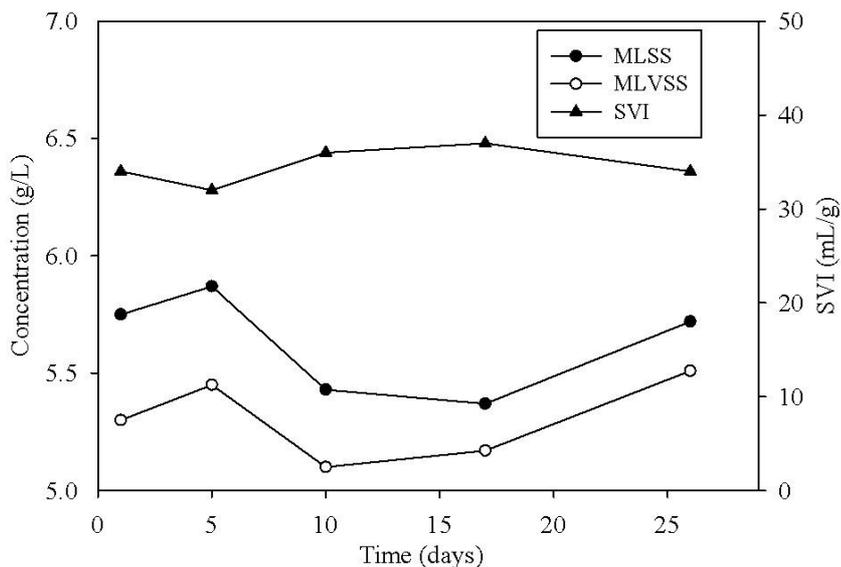
Figure 4.33 Variations of  $SVI_{30}$  and MLSS-MLVSS concentrations at a constant settling time (2 min) during operation in Set-3
