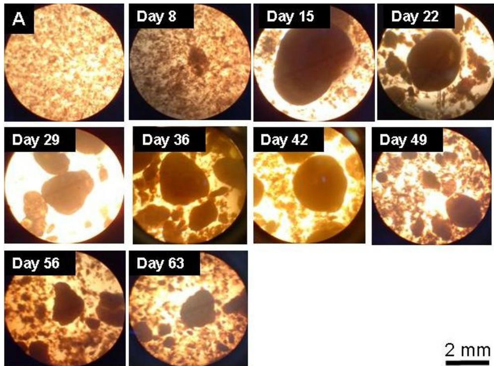
Figure 4.25 Evolution of flocs and granules during the operational period in R2 (aerobic-anoxic) in Set-2 (A: images taken at the end of the acclimation period)
