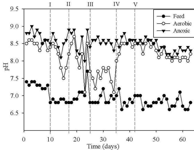
Figure 4.15 pH variations in R2 (aerobic-anoxic) during operation in Set-2 (-o- aerobic period -▼- anoxic period)
