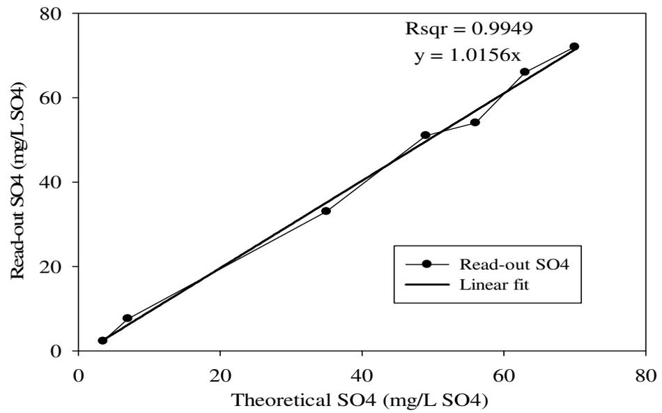
Figure B. 6 Calibration curve for SO<sub>4</sub><sup>2-</sup> range of 2-70 mg/L
