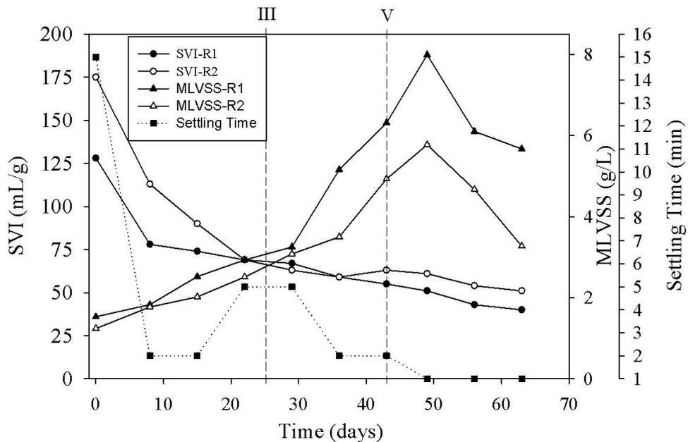
Figure 4.28 Variations of  $SVI_{30}$ , MLVSS concentrations inside the reactors and settling time during granulation in Set-2
