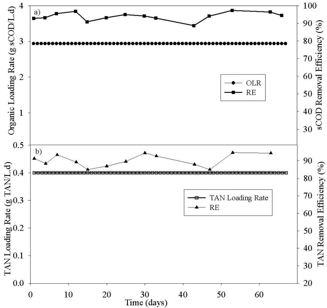
Figure D.1 Removal Performances for 67 days of operation under steady conditions
