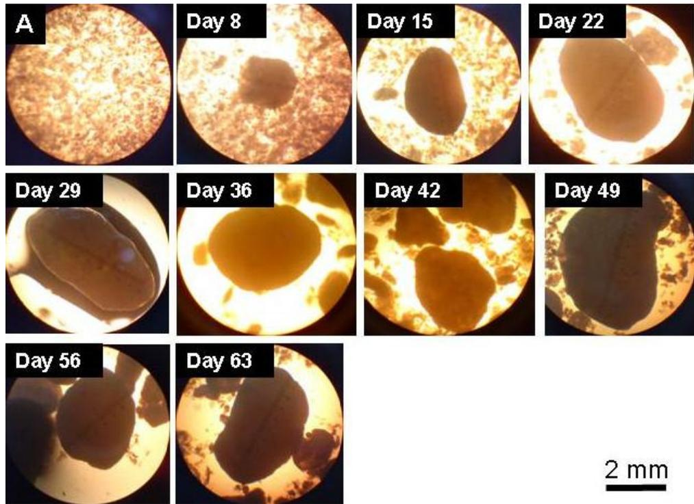
Figure 4.24 Evolution of flocs and granules during the operational period in R1 (anoxic-aerobic) in Set-2 (A: images taken at the end of the acclimation period)
