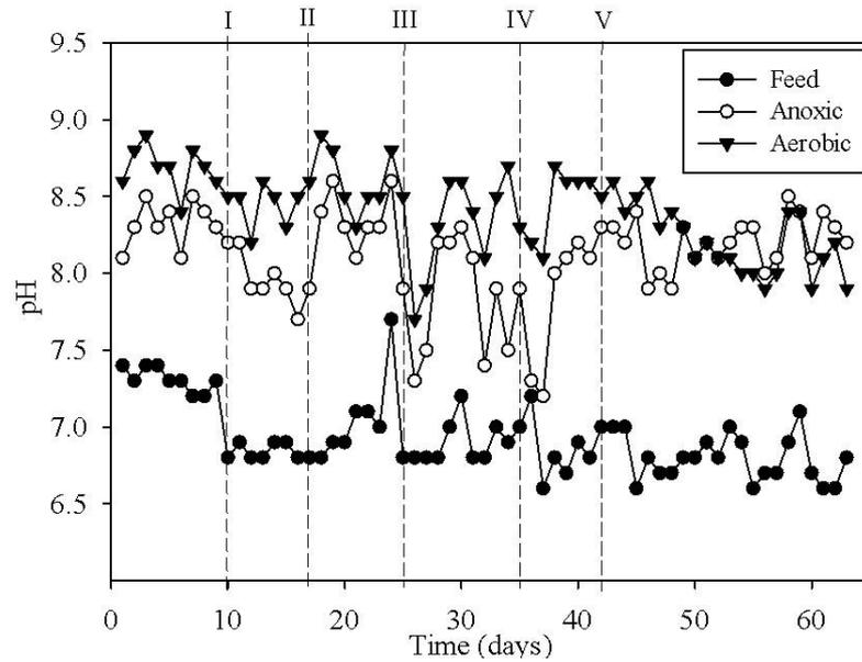
Figure 4.14 pH variations in R1 (anoxic-aerobic) during operation in Set-2 (-o- anoxic period -▼- aerobic period)
