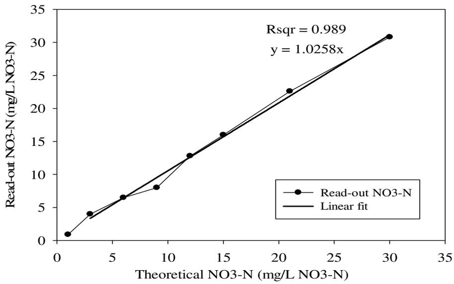
Figure B. 4 Calibration curve for NO<sub>3</sub>-N range of 0-30 mg/L
