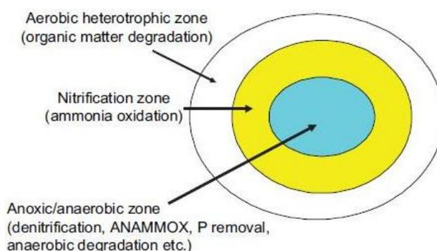
Figure 2.4 Conceptual aerobic granule structure (Gao et al., 2011)
