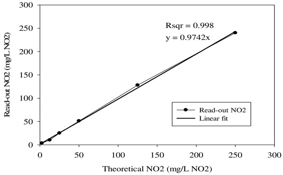
Figure B. 5 Calibration curve for NO<sub>2</sub> range of 0-250 mg/L
