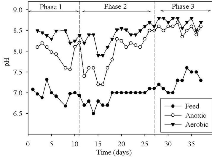
Figure 4.1 pH variations of R1 during operation (MBS) in Set-1 (-○- anoxic period -▼- aerobic period)
