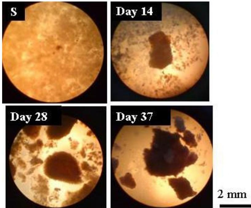
Figure 4.5 Microscopic view of sludge in R1 in Set-1 (S: Seed Sludge)
