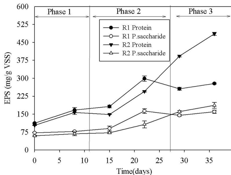
Figure 4.9 Variations in the EPS contents of the granules developed during operation in Set-1
