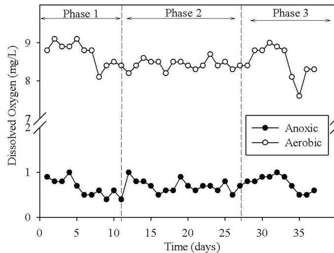
Figure 4.4 DO concentrations in R2 during operation in Set-1 (-●- anoxic period -○- aerobic period)
