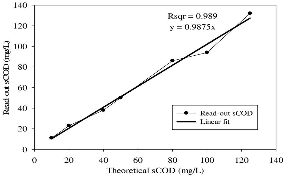
Figure B. 2 Calibration curve for sCOD range of 0-150 mg/L
