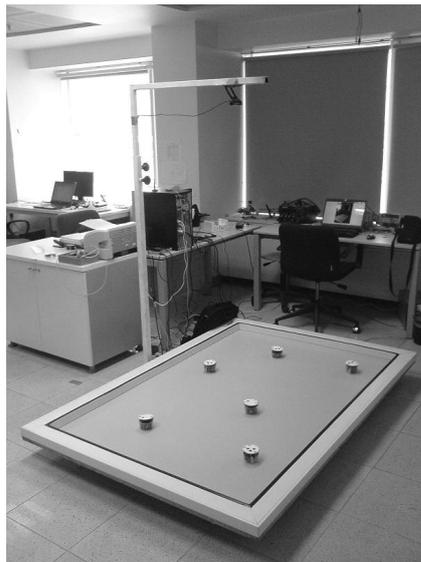
Figure A.1: Experimental setup consisting of an arena, robots, PC and overhead camera.
