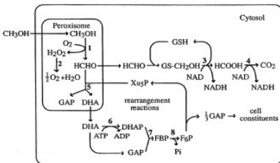
**Figure 2.5** Methanol utilization pathways in *P.pastoris*. Enzymes indicated by numbers: 1- AOX; 2- Catalase; 3- formaldeyhde dehydrogenase; 4- formate dehydro-genase; 5-dihydroxyacetone synthase;6- dihydroxyacetone kinase; 7- fructose 1,6 biphosphate aldolase; 8-frustose 1,6-biphosphophatase (Cereghino and Cregg, 2000).
