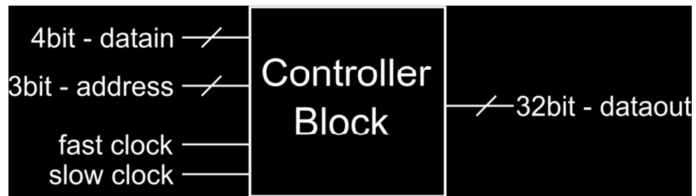
Figure 3.12: Input and output configuration of controller block.
