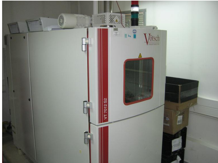
Figure 3.11. Thermal shock test chamber used by Arçelik.
