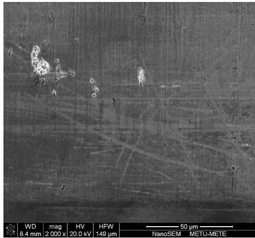
Figure B.3. Alloy with Sn-3.7Ag-0.9Cu composition before thermal shock.
