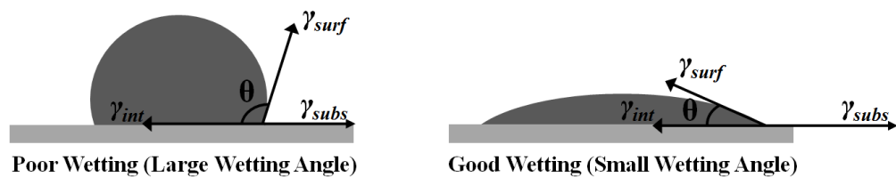
Figure 2.25. Poor and good wetting conditions.
