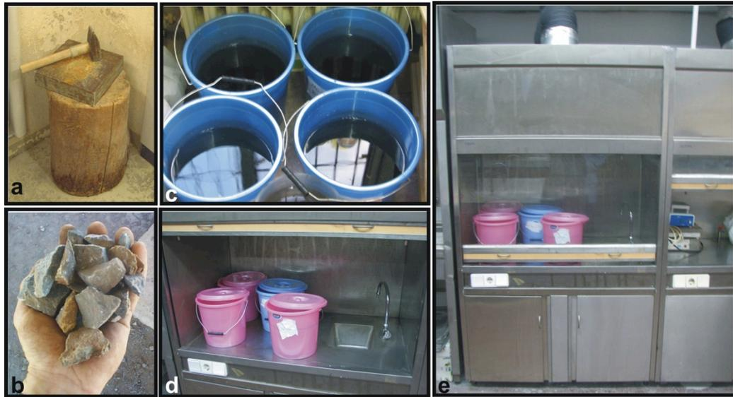
Figure 7.10. a-b. A calcareous rock sample broken into small pieces, c-e. digestion of carbonate by acid solution.
