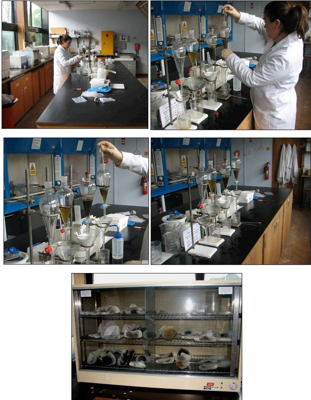
Figure 7.13. Concentration of conodont elements using Sodium Polytungstate heavy liquid.
