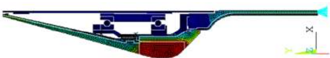
Figure 2-5. Temperature Distribution of the Tail Section
