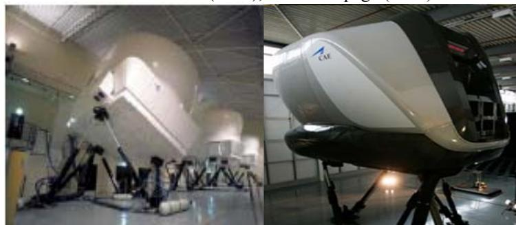
**Figure 2.1 Full Flight Simulators (FFS)**
