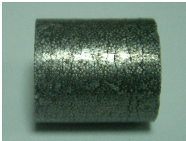
Figure 3.6 The radial cracks formed vertical to the direction of pressing.
