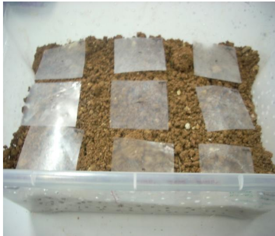
Figure 13: A photo from soil burial treatment
