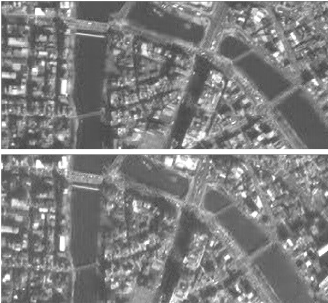
Figure 7.5. Compression artifacts observed in the ALOS Hiroshima stereo pair. The artifacts are visible in the low contrast regions (the river and shadows).
