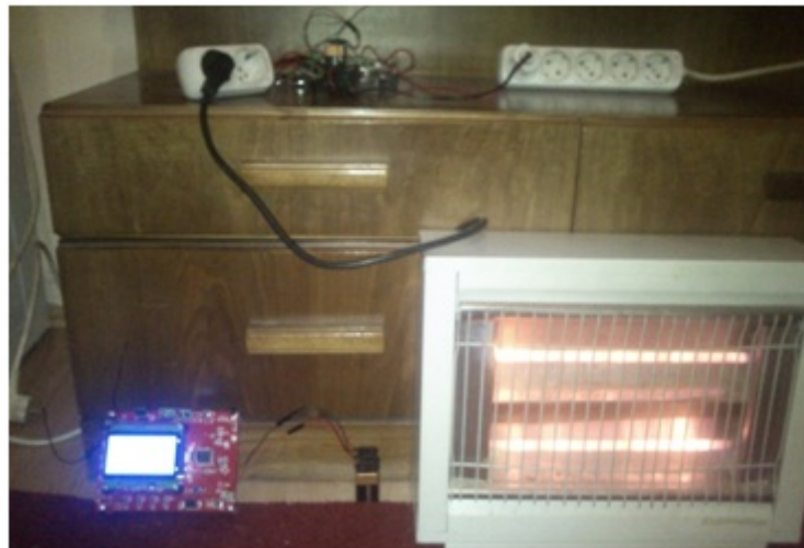
Figure 4.24: Test setup for electric heater current harmonics
