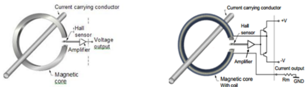
Figure 2.12: (a) An open loop Hall effect transducer (b) A closed loop Hall effect transducer
