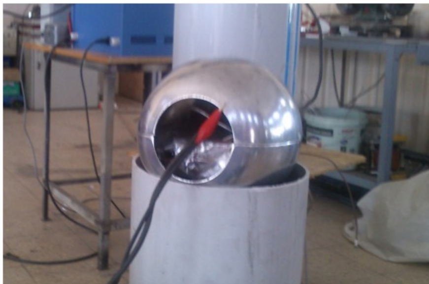
Figure 4.27: Faraday caging around data-acquisition card
