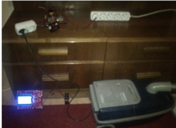
Figure 4.22: Test setup for testing vacuum cleaner current harmonics
