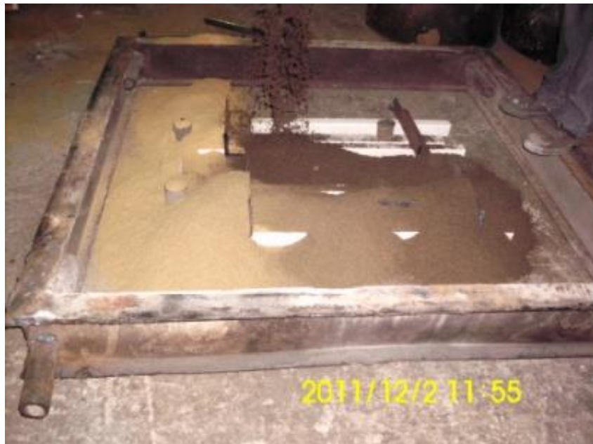
Figure 4.2 The Filling of the Drag with Sand
