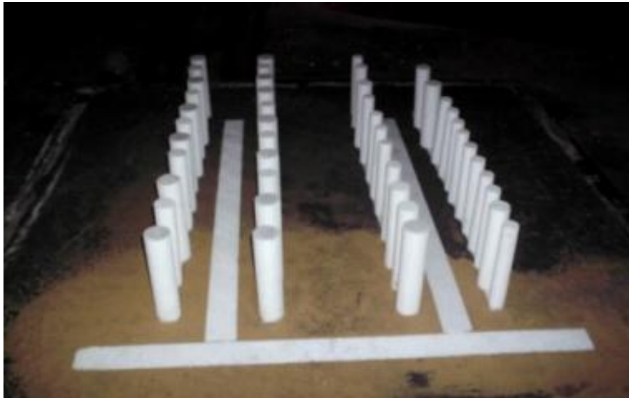
Figure 4.3 The Patterns of the Billets Placed in the Middle Flask
