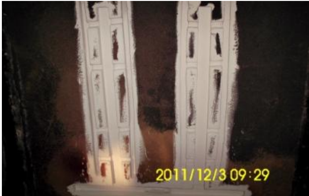
Figure 4.7 Painted Cavity of Gating System (Lowest Flask)
