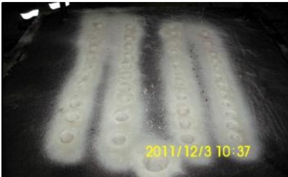
Figure 4.8 The view of the Cope after Painting
