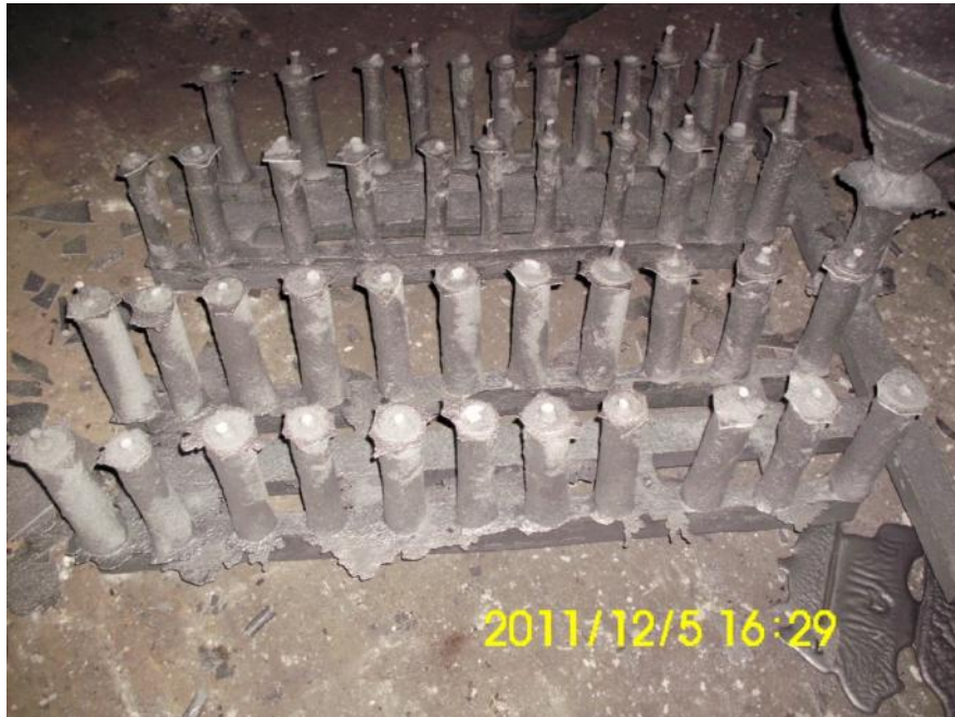
Figure 4.12 Specimens after shakeout
