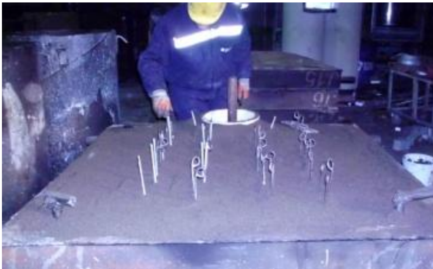
Figure 4.6 Molding of Cope
