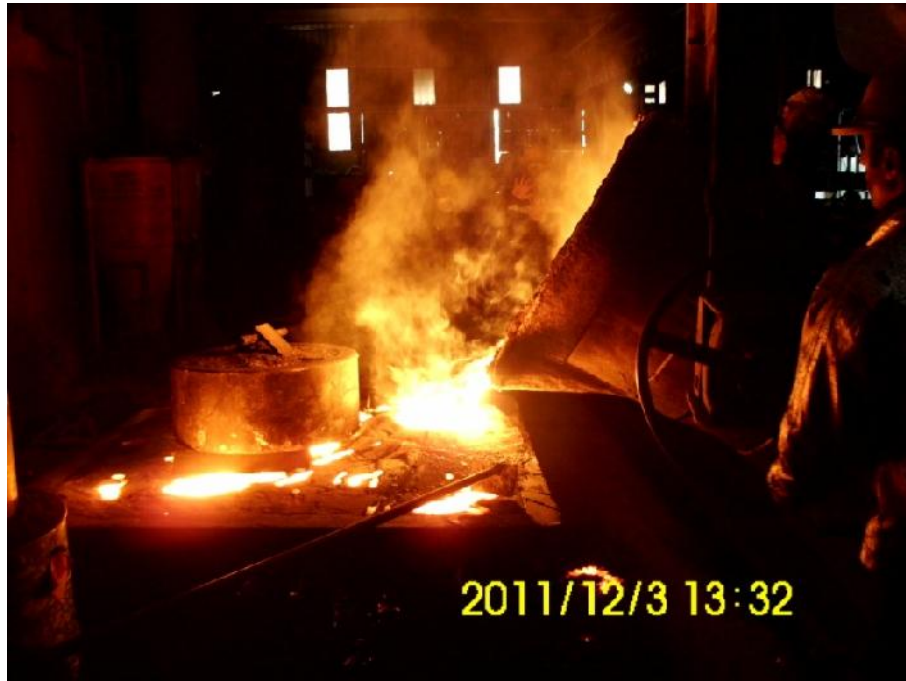
Figure 4.11 Pouring of tool steel into the mold
