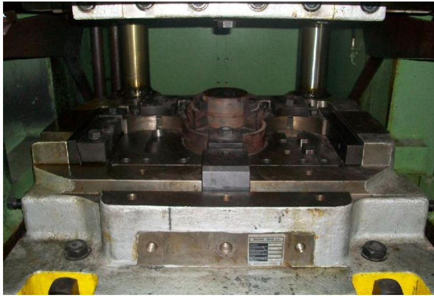
Figure 6.3 Lower Die Assembly of the Forging Press
