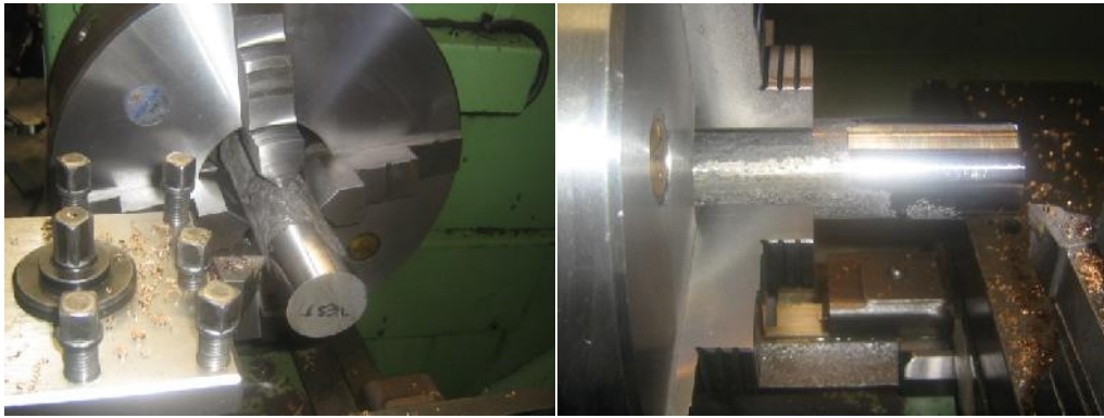
Figure 6.1 Turning Operation of the Specimens
