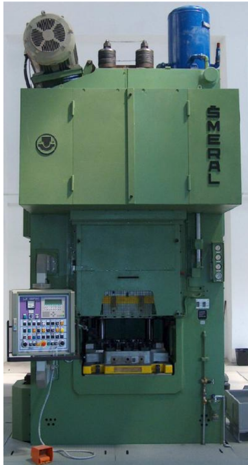
Figure A.1 Smeral 10 MN Mechanical Press in METU-BILTIR Center Forging Research and Application Laboratory
