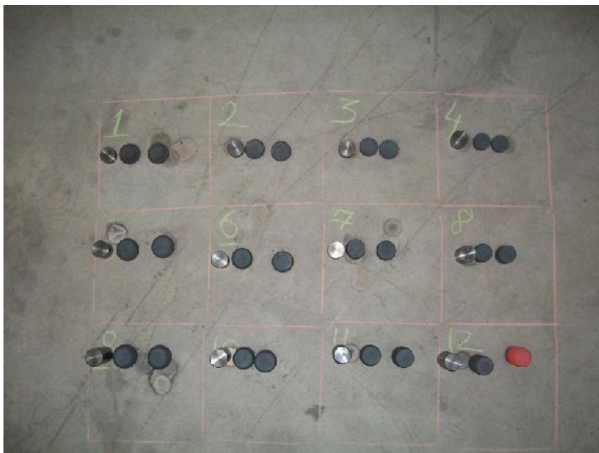
Figure 6.7 Grouped Billets After Forging
