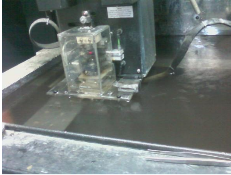
Figure 7.4 V- Notch Machining by Electrical Discharge Machining
