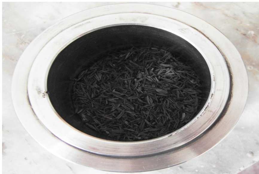
Figure 3.2 Coked rice husks inserted into the milling bowl
