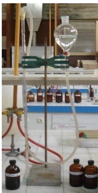
Figure 3.1. Gas volume analysis apparatus for anaerobic batch reactors
