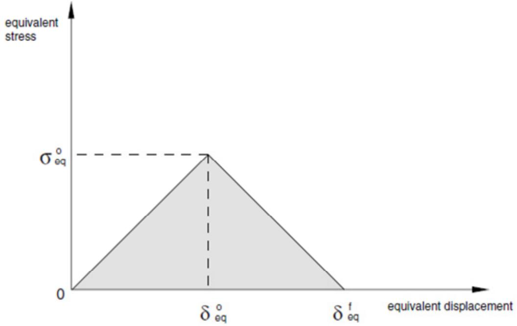
Figure 22. Equivalent Stress-Equivalent Displacement Curve [36]
