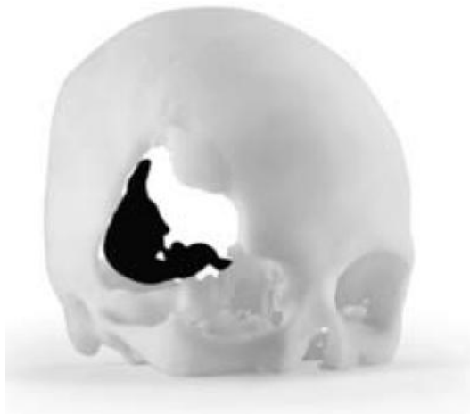
Figure 2.19 Tumor illustrated in a different material inside the skull (Gibson, Rosen, and Stucker 2009, 388)
