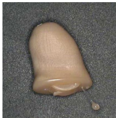
Figure 2.17 Rapid manufactured hearing aid (Gibson, Rosen, and Stucker 2009, 366)
