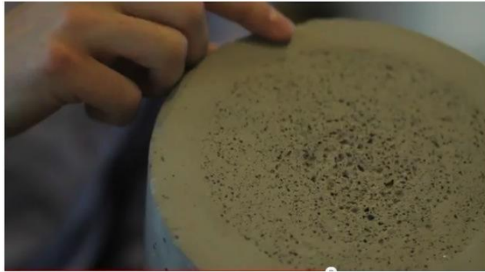
Figure 2.25 Concrete column section 3D printed with variable density (Chandler 2012)
