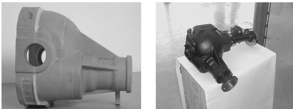
Figure 2.5 3D printed (left) and manufactured (right) differential housing by investment casting (Dimitrov, Schreve, and Beer 2006, 140)
