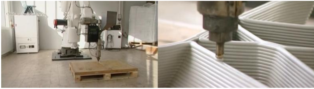
Figure 3.2 5-axis robot and its extruder head used in the manufacturing process of Endless series furniture (Vander Kooij 2012)
