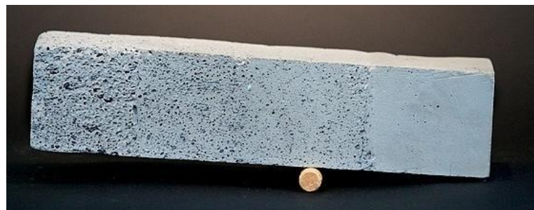
Figure 2.26 Concrete block 3D printed with variable density (Chandler 2012)
