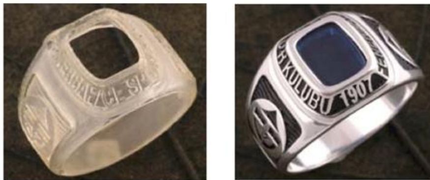
Figure 2.7 Pattern (left) and the manufactured (right) ring via SLA (Negis 2009)
