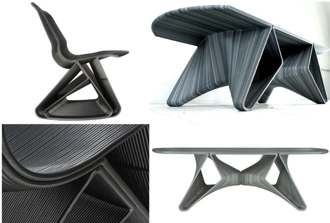
Figure 3.1 Endless series furniture manufactured with FDM (Vander Kooij 2012)
