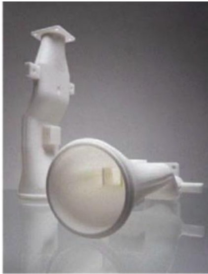
Figure 2.9 Cooling ducts with rapid manufacture (Levy,Schindel, and Kruth 2003)
