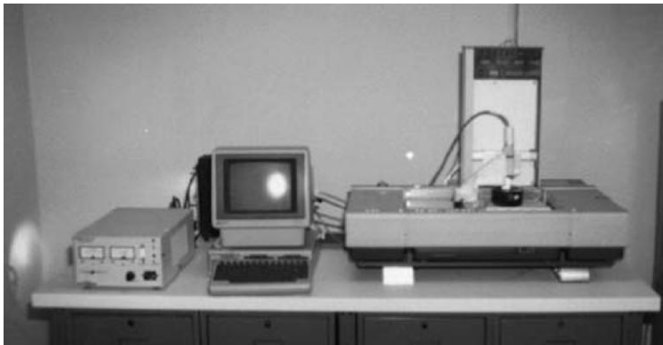
Figure 2.1 The first additive manufacturing technology, patented by Hull (Gibson, Rosen, and Stucker 2009, 34)
