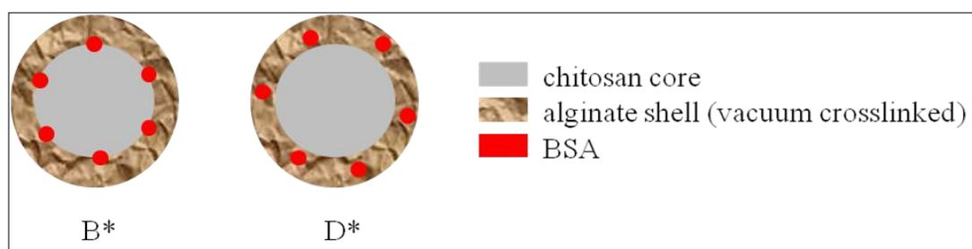
**Figure 2.3.** Schematic representation of loading models with vacuum crosslinked alginate layer.
