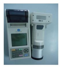
Figure 10 Minolta CR-410 Colorimeter
